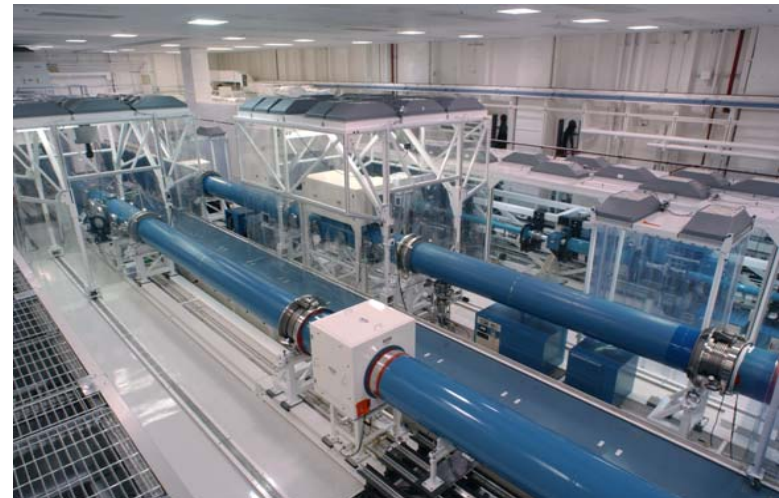
Z-Beamlet multikilojoule laser facility
