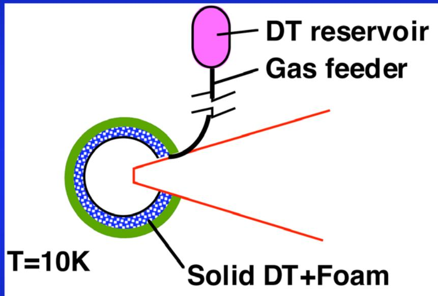
We are going to use foam technique to support solid DT layer and a gas feeder to load fuel in the shell.
