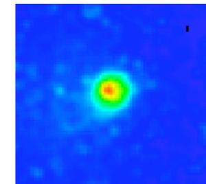
Spot size is  $30\mu\text{m}\phi$
