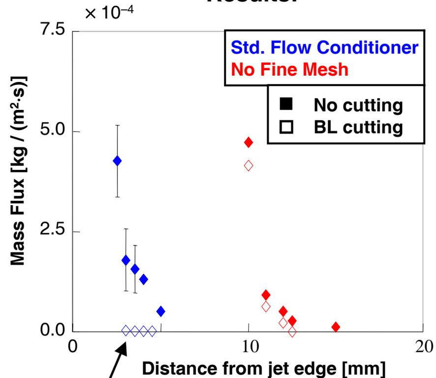
**Flow conditioning and boundary layer trimming are needed to suppress drop ejection**
