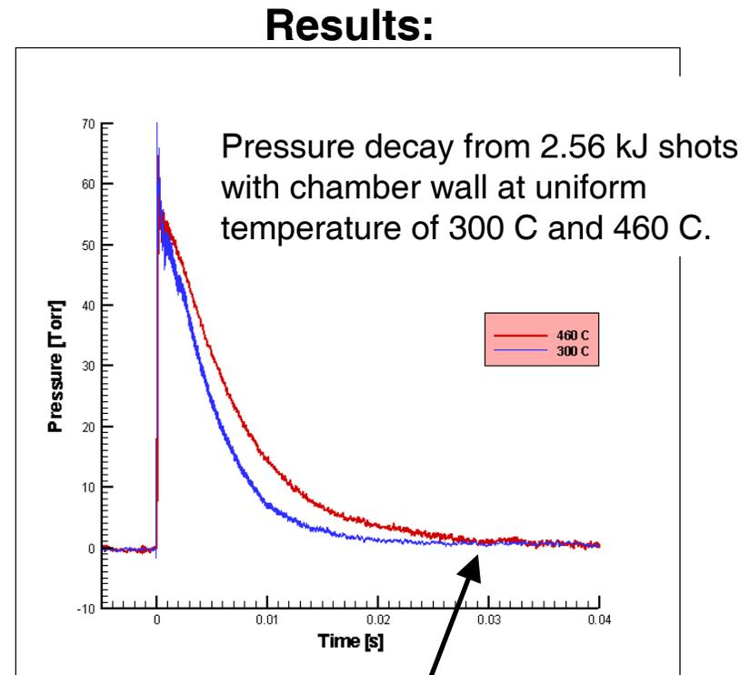
**Transient condensation of superheated LiF vapor is completed in about 30 ms. This scales to <100 ms in IFE chamber, compatible with allowed clearing period.**
