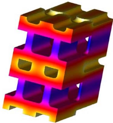
Temperature distribution in heat exchanger element
