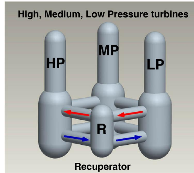
Adapting GA's Gas Turbine-Modular Helium Reactor (GT-MHR) Power Conversion Unit to fusion (vessels are ~ 30 m high)
