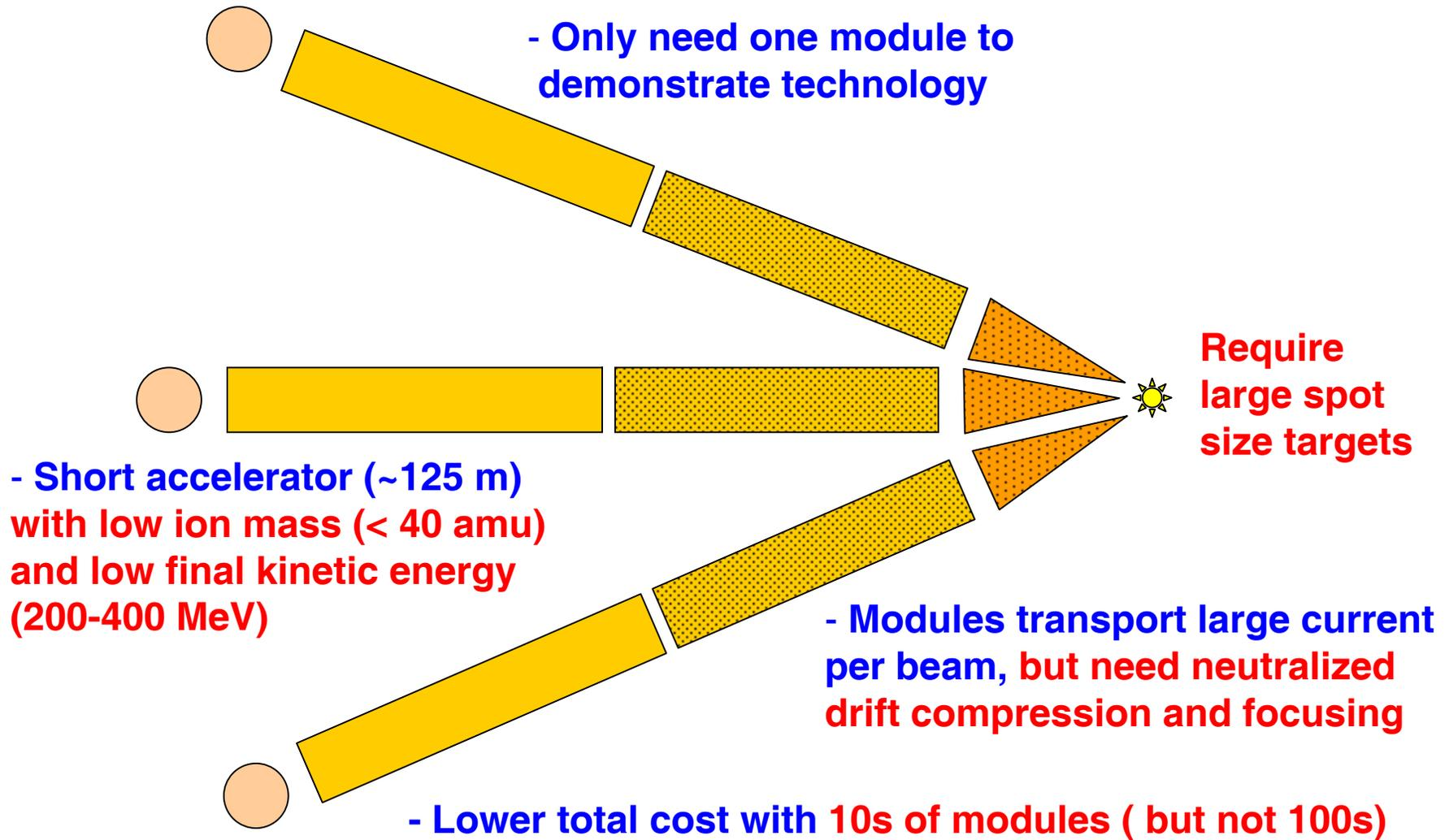
**Neutralized drift compression/focusing + hybrid targets may reduce costs by ~50% for both conventional multiple-beam quadrupole and modular solenoid driver options for IFE**
