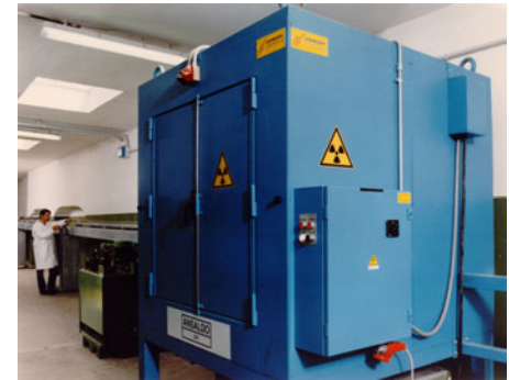
Butt weld x-ray inspection
