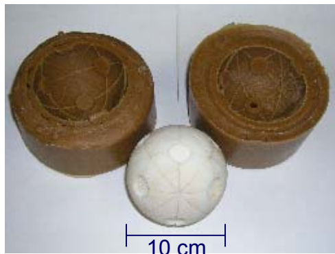
1. Mold produced from rapid prototype model
