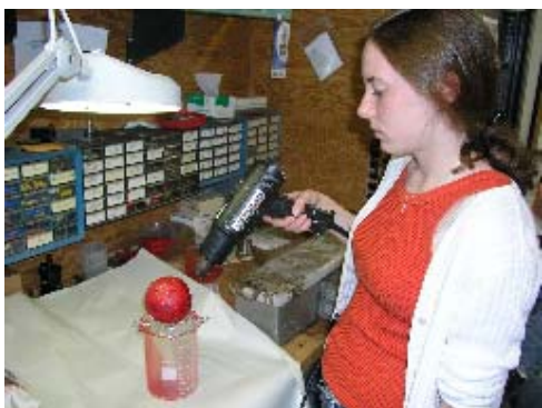
5. Wax form melted away at ~80 °C
