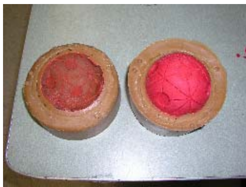
2. Wax poured into mold
