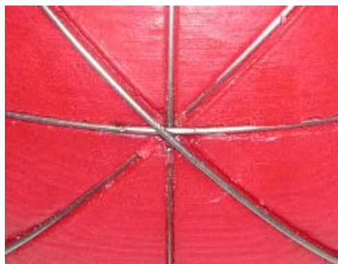
4. Wires spot welded at junctions
