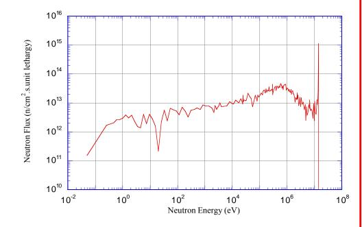
Large dip in spectrum around 20 eV due to giant  $^{186}$ W (n, $\gamma$ ) resonance
