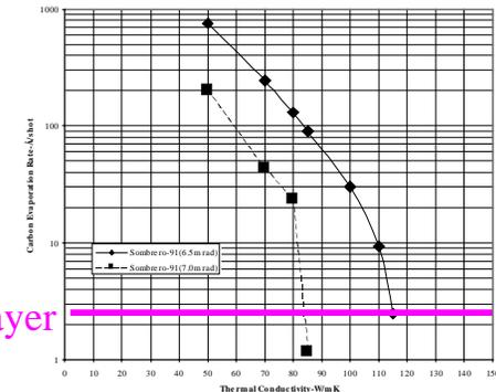
**Status:** BUCKY (continuum) calculations show that it is possible to get wall erosion per shot of less than 1 mono-layer of material loss per shot, but what does that mean?
