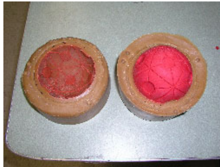
2. Wax poured into mold
