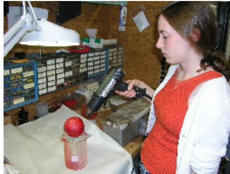
5. Wax form melted away @100C
