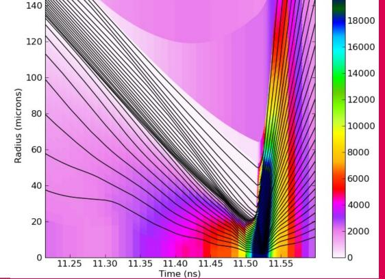
Ion Temperature Sudden acceleration when slabs impact
