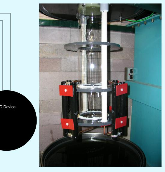
•High voltage buffer circuit (shown left) decreases instability, and new insulators (right) enable high voltage connection in plasma
