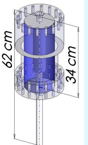
•Combined system has been operated up to 170 kV, up to 75 mA, and at pressures as low as 3 mPa
