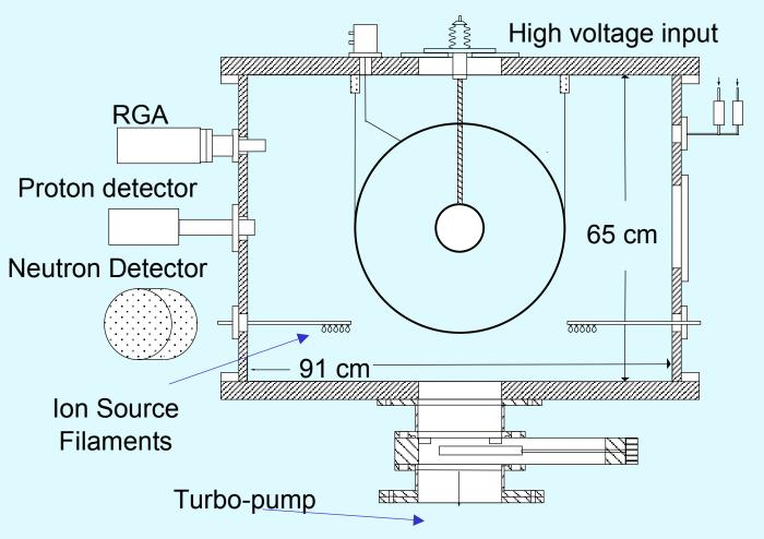
•<sup>3</sup>He-<sup>3</sup>He fusion requires high ion energies, which necessitates high cathode voltages and low neutral gas pressure
