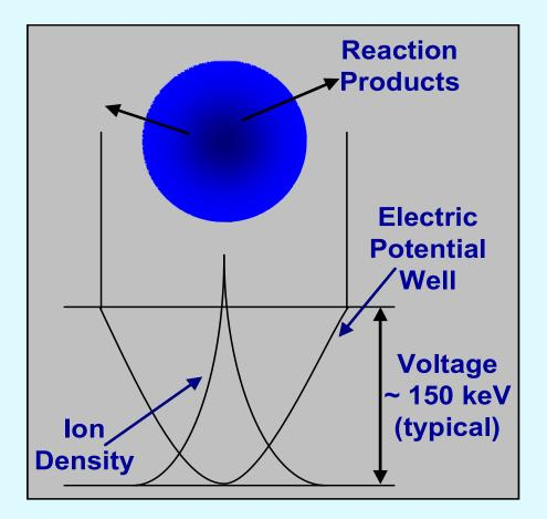
•IEC technology confines ions in an electrostatic potential well
