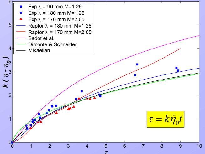
Results from simulations with Raptor (2D) are also shown above, At left, the dimensionless amplitude  $\eta$  of the interface (excluding wall effects) from simulations and experiments at various shock strengths (M) is plotted on a dimensionless timescale, with analytical model predictions.
