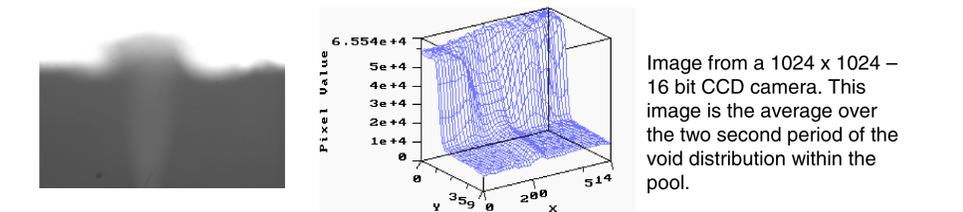
Image from a 1024 x 1024 - 16 bit CCD camera. This image is the average over the two second period of the void distribution within the pool.
