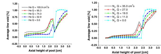
From the images above the line average void distribution in the pool can be calculated using the calibration curve relating the pixel value with void.
