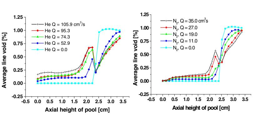
Plots show the average void produced for different volumetric flow rates. As the flow increases the amount of liquid metal lifted by the jet increases.
