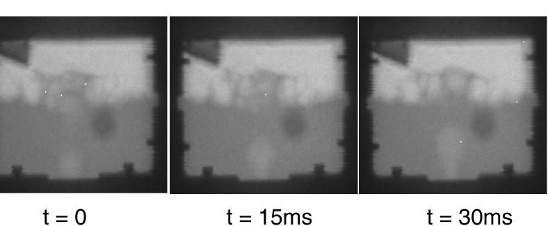
Helium injection at 23 cm<sup>3</sup>/s into NaK with no magnetic field. There is significant surface agitation and bubbling.
