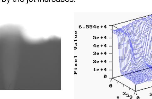
Image from a 1024 x 1024 -16 bit CCD camera. This image is the average over the two second period of the void distribution within the pool.
