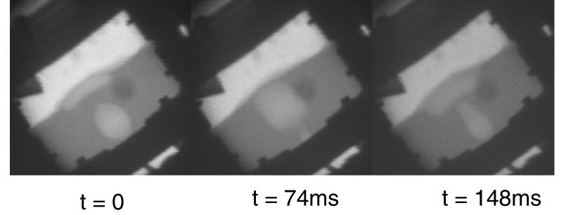
Injection of helium at 23 cm<sup>3</sup>/s with a 10kG magnetic field. The pool becomes very calm and the bubbles become larger and wider with a lower frequency of departure. The bubbles are elongated when they leave the pool surface (the image was rotated due to effects of B field on CCD array).
