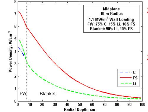
Peak surface heat flux at midplane =0.37 MW/m<sup>2</sup> • Drops to 0.13 MW/m<sup>2</sup> at top/bottom with an average value of 0.26 MW/m<sup>2</sup> > Peak neutron wall loading at midplane =1.09 MW/m<sup>2</sup> • Drops to 0.39 MW/m<sup>2</sup> at top/bottom with an average value of 0.77 MW/m<sup>2</sup>
