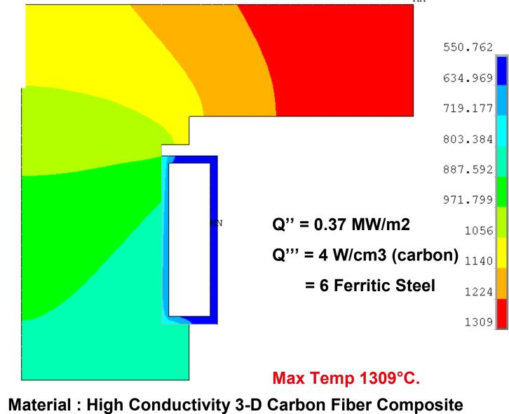
Ferritic Steel Coolant Rail, Lithium Coolant
