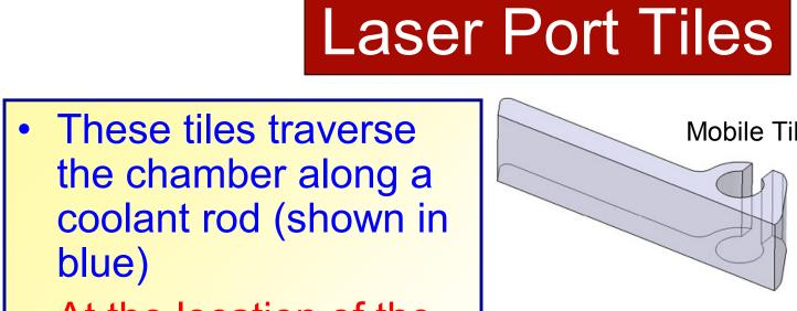
At the location of the laser ports, the tiles will rotate around the coolant rod by following a guiding rail on the coolant rod
