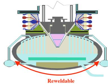
Mechanical attachments or other means for wall assembly should be considered for chamber top and behind jets
