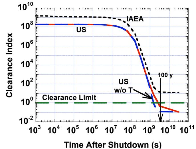
RTL waste could be stored for 50-100 y after plant decommissioning, then cleared (released to commercial market for reuse)
