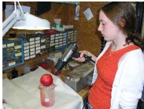
5. Wax form melted away at \sim 80^\circ\text{C}
