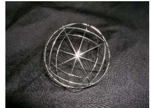
6. Finished grid cathode
