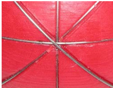
4. Wires spot welded at junctions
