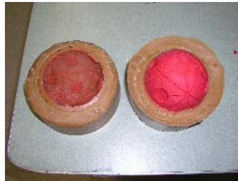
2. Wax poured into mold
