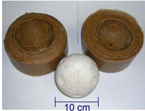
1. Mold produced from rapid prototype model
