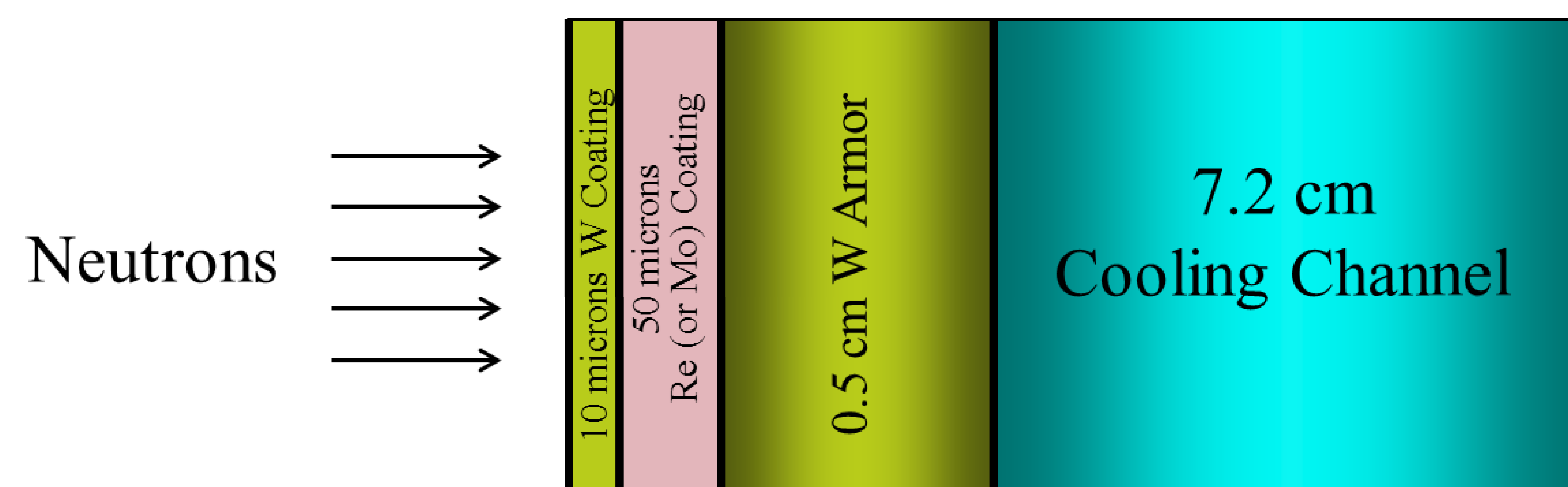
Radial build of divertor model for WDR calculations given Re and Mo coatings of thicknesses varying from one to 50 microns.
