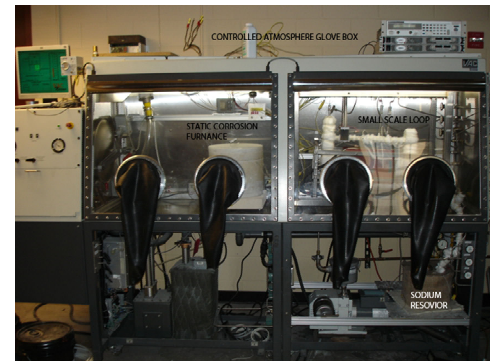
The ceramic testing glove box houses a static testing system and a 1+ gallon flowing loop.
