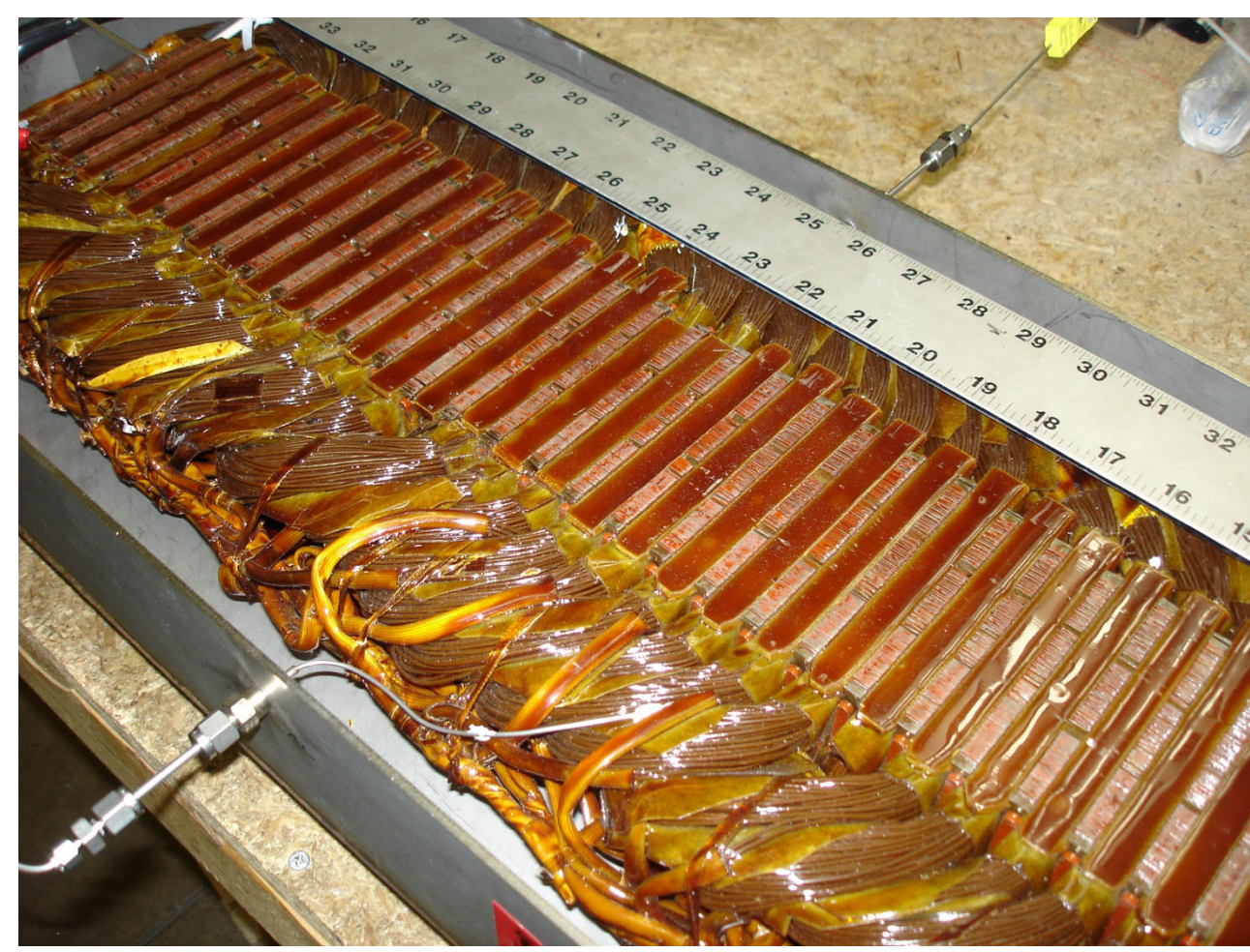
The coils of the FLIP are impregnated with an epoxy that can withstand temperatures up to 180°C. The coils are also oil resistant.
