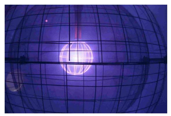
Cathode Voltage=55 kV Cathode Current=60 mA Pressure= 1 mTorr
