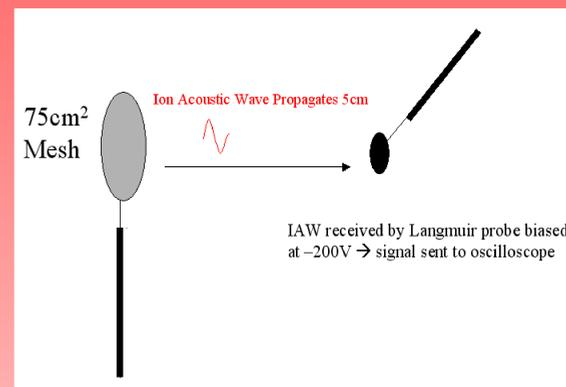
This figure portrays the experimental setup used to verify the molecular ion concentrations calculated to exist in the IEC source region. Excitation signals on the 75cm<sup>2</sup> mesh were kept to ~2Vpp to ensure the propagation of linear IAW waves.
