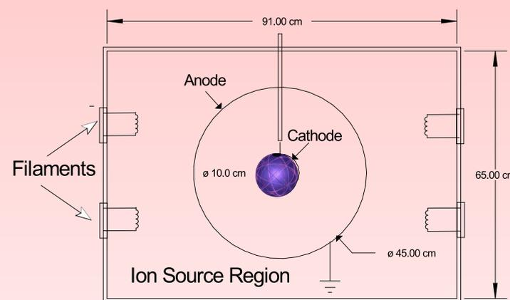
This schematic shows the geometry of the UW-IEC Device
