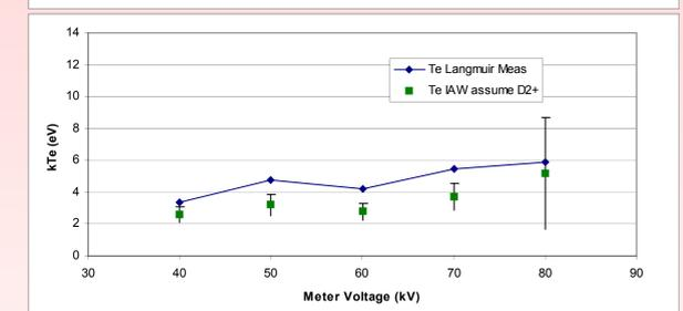
Comparison of IAW calculated electron temperatures assuming  $D_2^+$  and  $D_3^+$  plasmas (data points) with measured electron temperatures (solid lines). Indicates minimum  $D_3^+$  concentrations of 60%.
