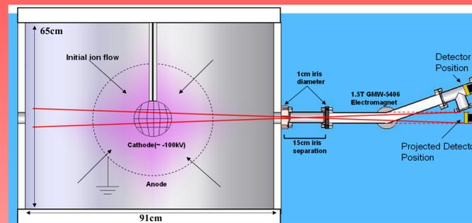
Figure 3: A schematic of the FIDO diagnostic is shown to illustrate the how the diagnostic geometry enhances the detection of fusion products with only parallel and anti-parallel velocity components.
