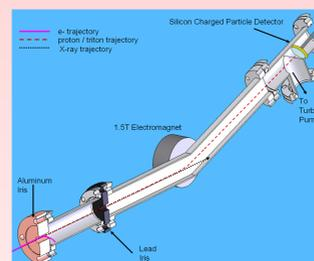
Figure 4: This schematic illustrates the trajectories taken by  $e^-$ 's, fusion products, and X-rays in the FIDO arm
