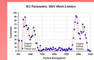
Figure 5: Above is a fusion product energy spectrum that shows both Doppler shifted tritons and protons from D-D fusion. Prior to the FIDO diagnostic this resolution was impossible, due to X-ray noise.
