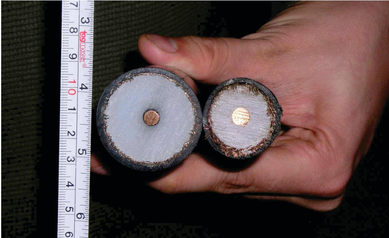
(New) 300 kVDC cable, left, and (current) 200 ,VDC cable, right
