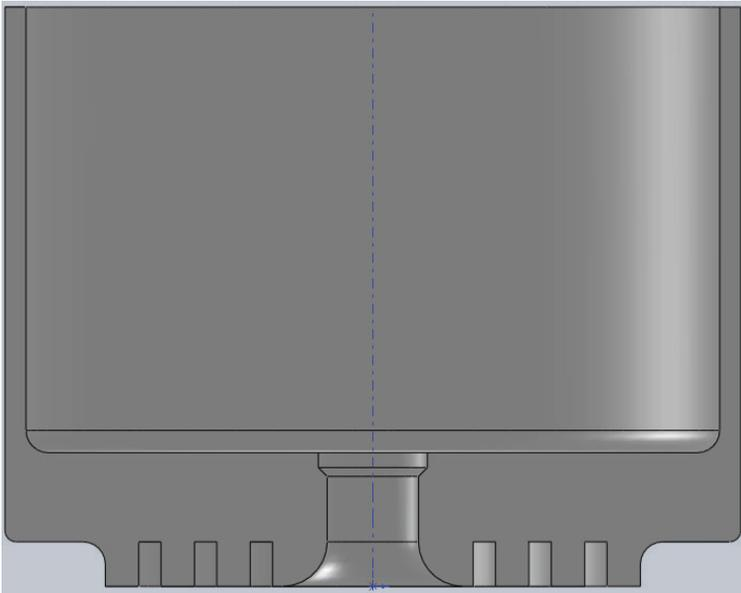
Quartz chosen for its high purity, tolerance of high temperatures (min 1000C), and high mechanical strength (1000psi tensile strength)
