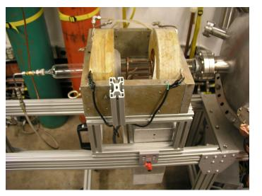
• Plasma densities in helicon sources can be increased by over 50% by changing the RF antenna from a Nagoya type III to a twisted Nagoya geometry [3]. An additional factor of 3-4 can be achieved by applying a non-uniform magnetic field instead of a uniform axial one [4]. These modifications will be tested in the near future to increase the extractable ion current.
