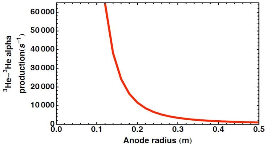
( $V_c=200$  kV,  $I_c=60$  mA,  $r_c=0.1$  m,  $r_a=0.2$  m)
