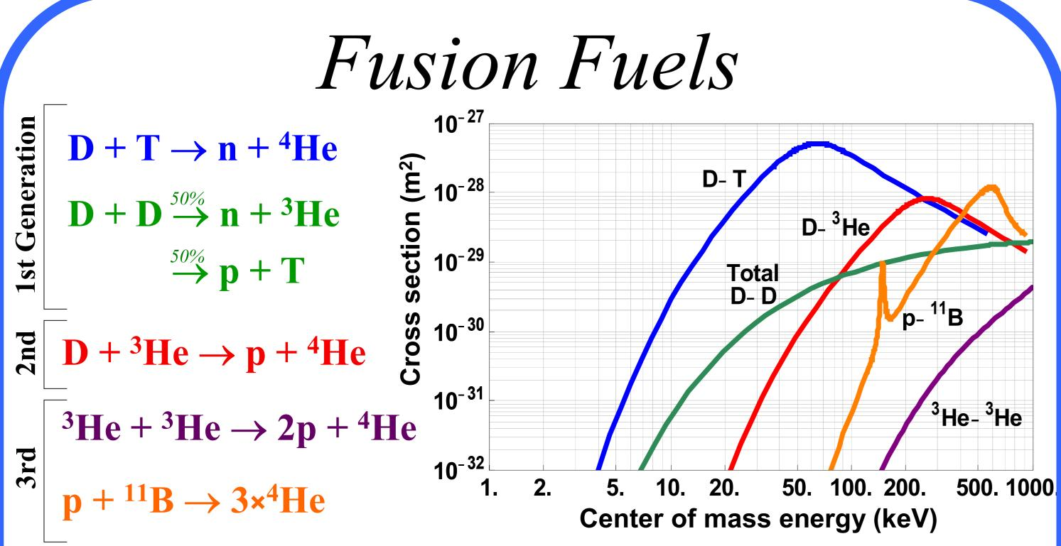
p = proton (hydrogen-1); D = deuterium (hydrogen-2); T = tritium (hydrogen-3);  ${}^{3}\text{He} = \text{helium-3}; {}^{4}\text{He} = \text{helium-4}; {}^{11}\text{B} = \text{boron-11}; n = \text{neutron}.$
