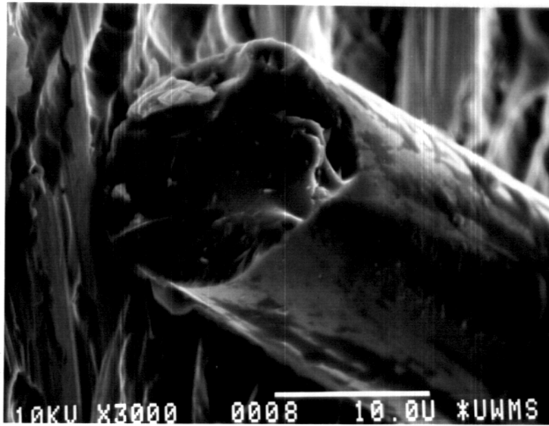
Fig. 2.5. Fatigue fiber fracture at 18,600 cycles for \sigma_m/\sigma_f = .40\% , \sigma_a/\sigma_f = 20\% .
