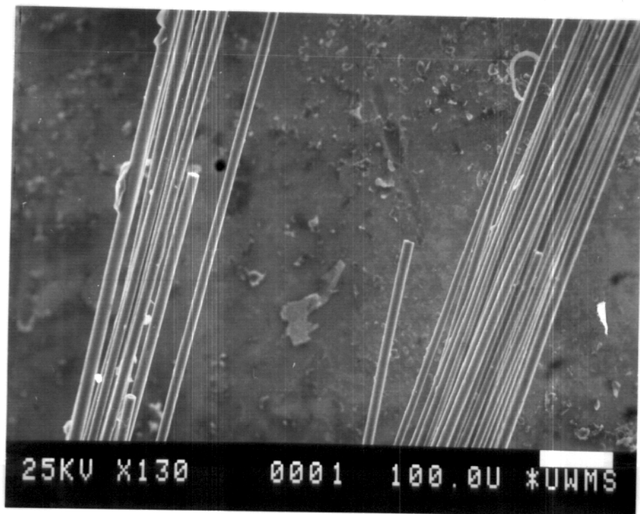
Fig. 5.1 Static tensile fracture of SiC fibers. Bar scale = 100 microns.
