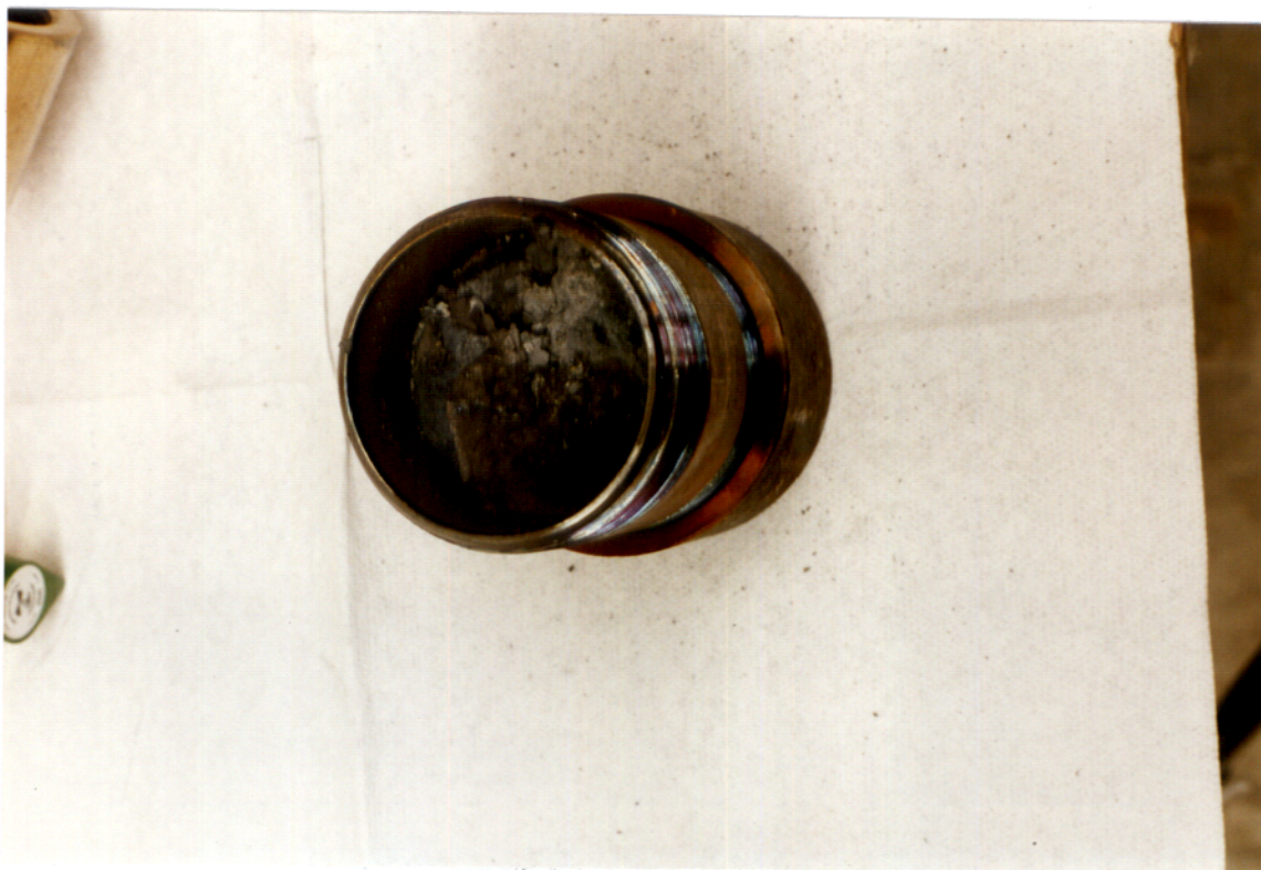
Figure 20. Body of the reactor used in the preliminary test A-123-1. Solidified alloy with flaky surface can be seen.
