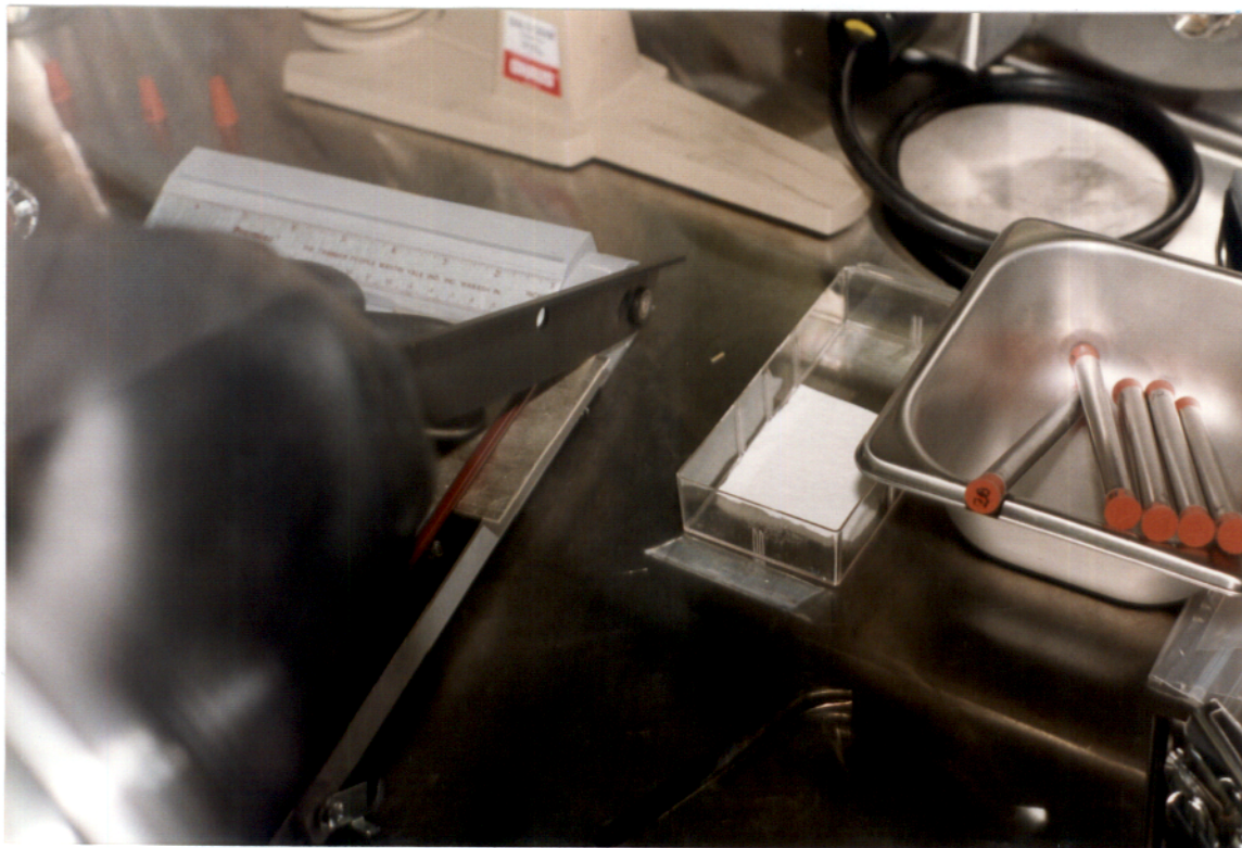
Figure 17. Start of cutting of strip of lithium foil in the glove box.
