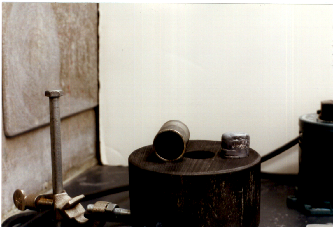
Figure 35. Sample of alloy from Batch No. A-123-1 resting on graphite heat sink. Also shown is the stainless steel mold.
