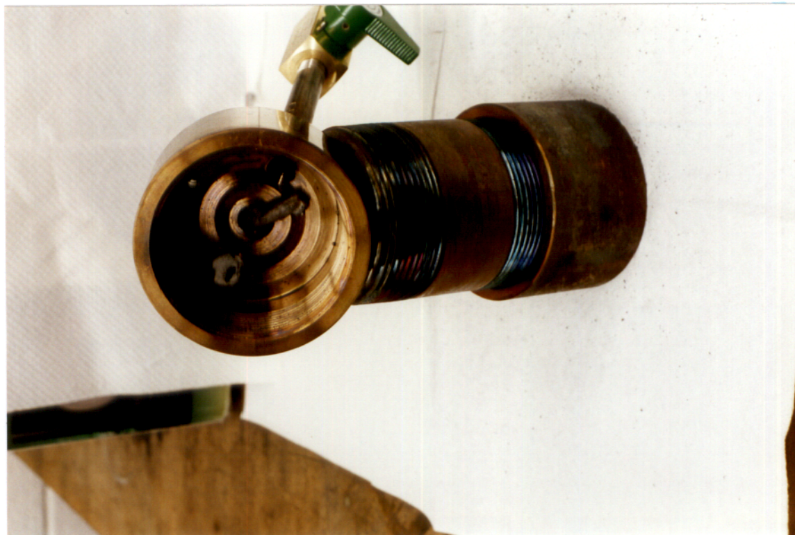
Figure 21. Disassembled reactor used in the preliminary test A-123-1. Upper pipe cap with retracted stirrer and thermocouple well rests on the body of the reactor shown in Figure 20.
