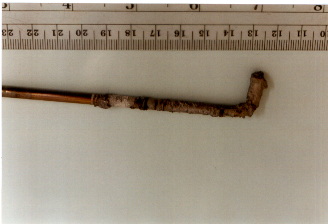
Figure 22. Stirrer after removal from the upper pipe cap shown in Figure 21. Note slag-like coating.
