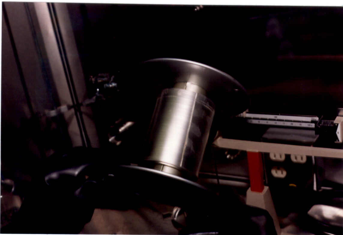
Figure 13. Lithium foil on spool, ready to be removed.
