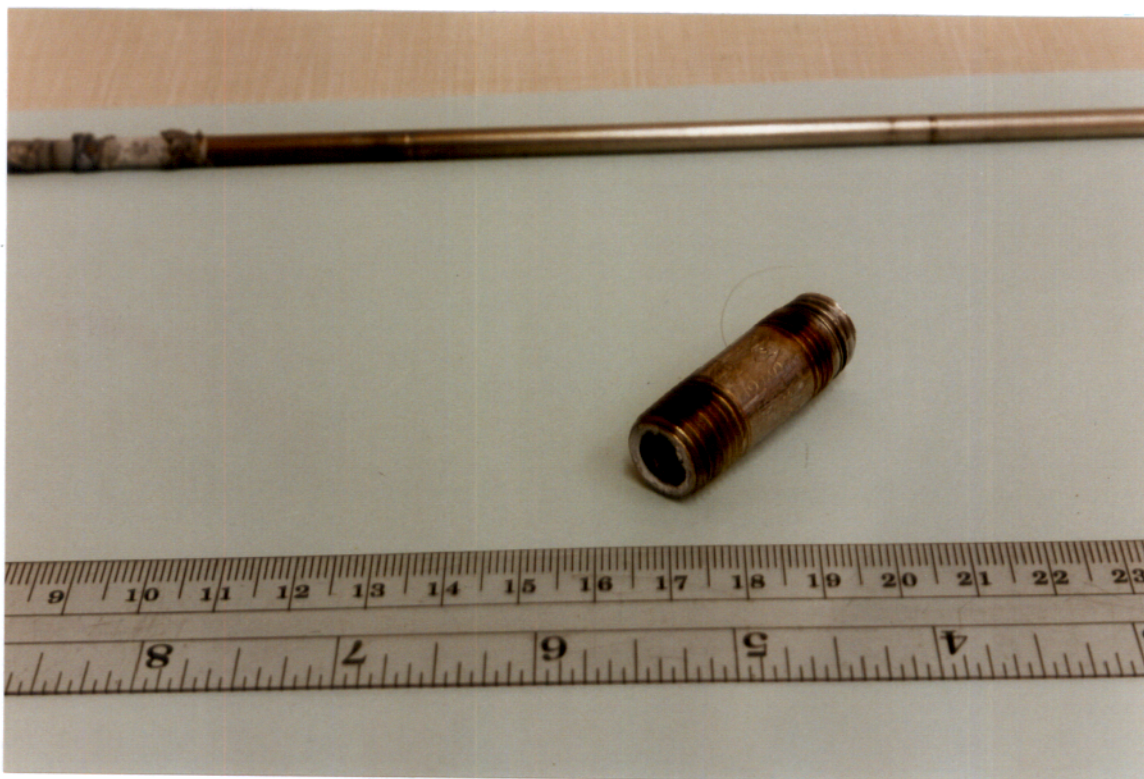
Figure 24. Outer end of partially plugged 1/4 in. pipe nipple removed from upper cap of the reactor shown in Figure 21. Note deposit of metallic lithium.
