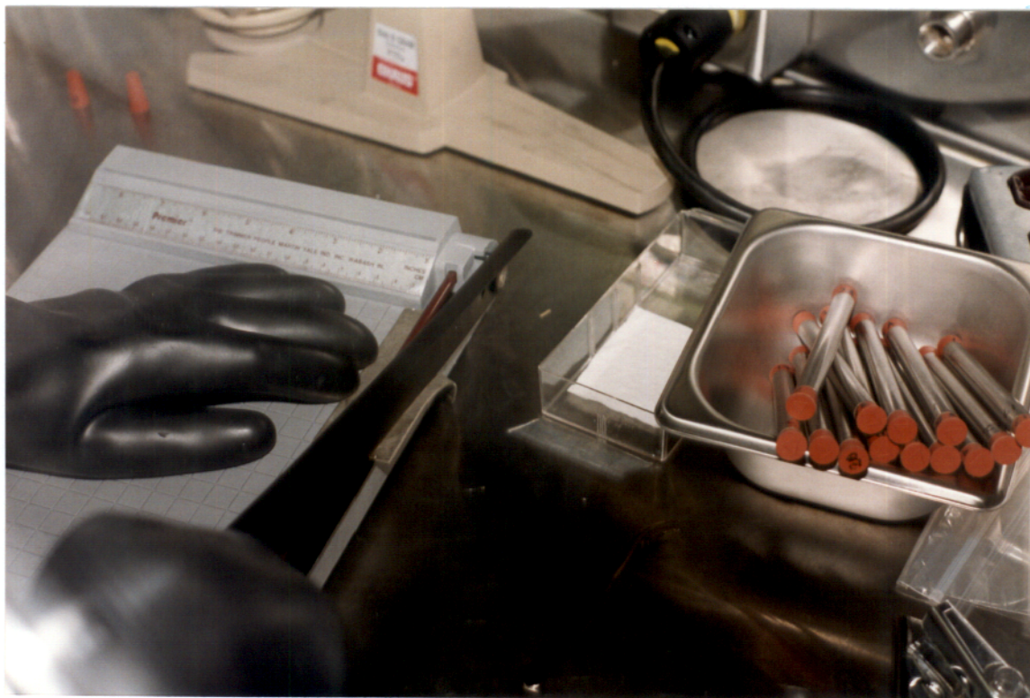
Figure 18. Nearly completed cutting of a strip of lithium foil. Note the curl imparted to the strip as it is being cut.
