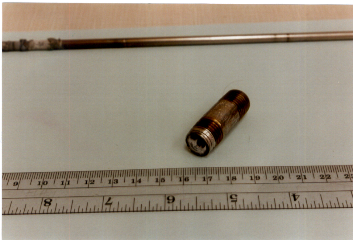
Figure 23. Inside end of partially plugged 1/4 in. pipe nipple removed from upper cap of the reactor shown in Figure 21. Note deposit of metallic lithium.
