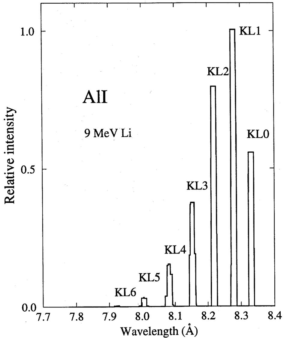
Figure 2. Computed relative intensities of Al  $K_{\alpha}$  satellite lines for AlII bombarded by 9 MeV  $\text{Li}^{+3}$  ions.
