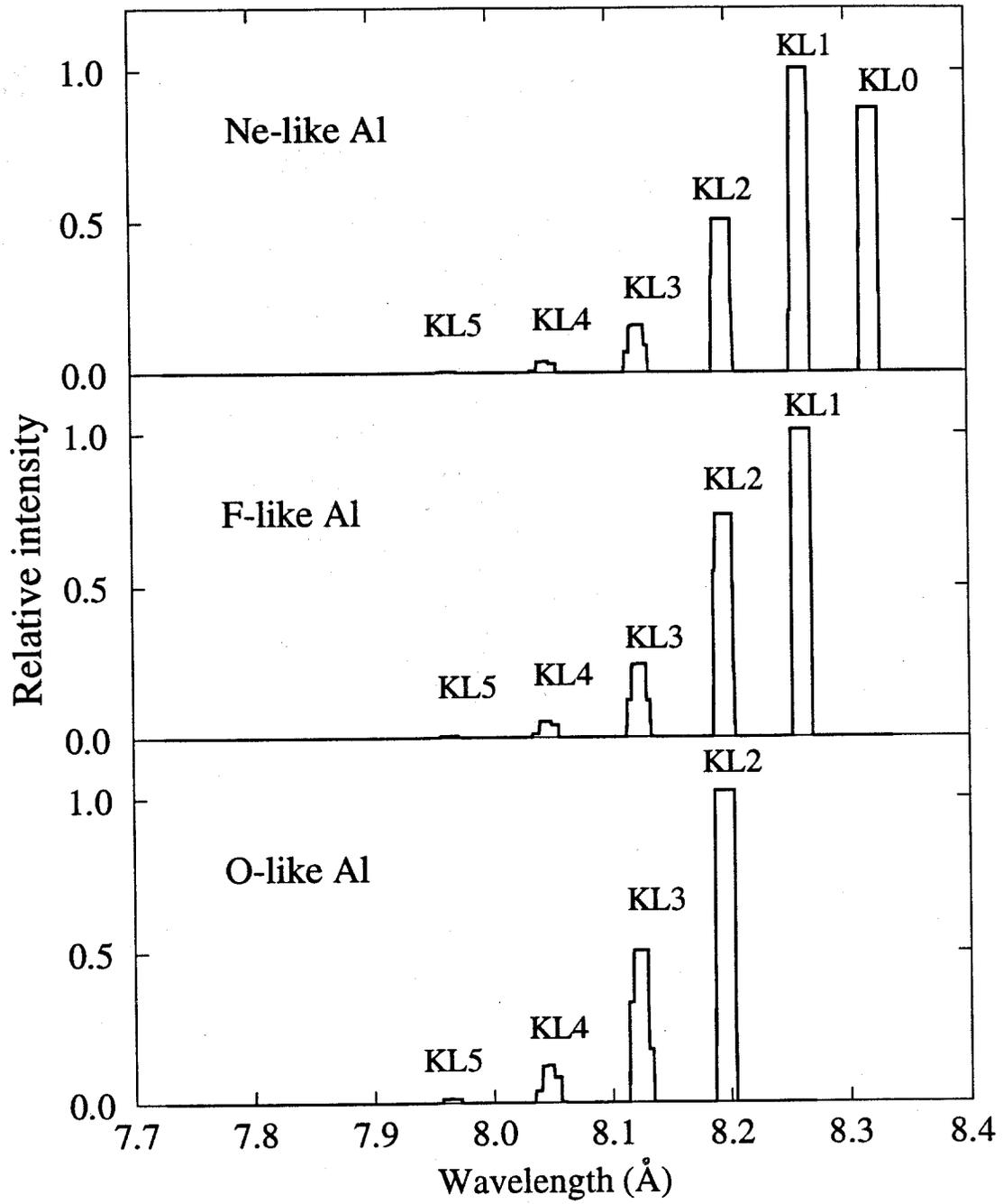
Figure 4. Computed Al  $K_{\alpha}$  satellite lines for Ne-, F-, and O-like Al ions by 9 MeV  $\text{Li}^{+3}$  bombardment.
