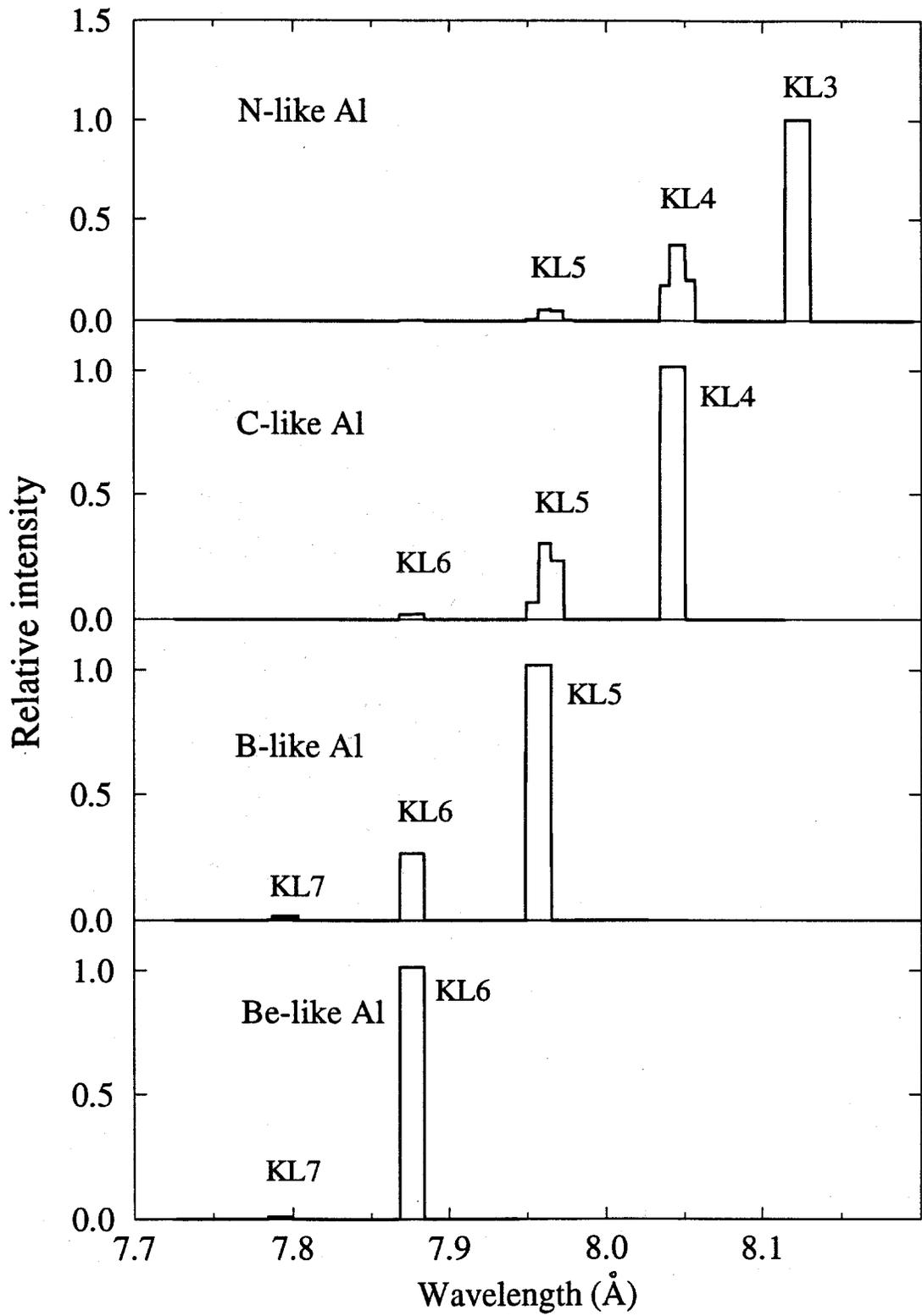
Figure 5. Computed Al  $K_{\alpha}$  satellite lines for N-, C-, and B-like Al ions by 9 MeV  $\text{Li}^{+3}$  bombardment.
