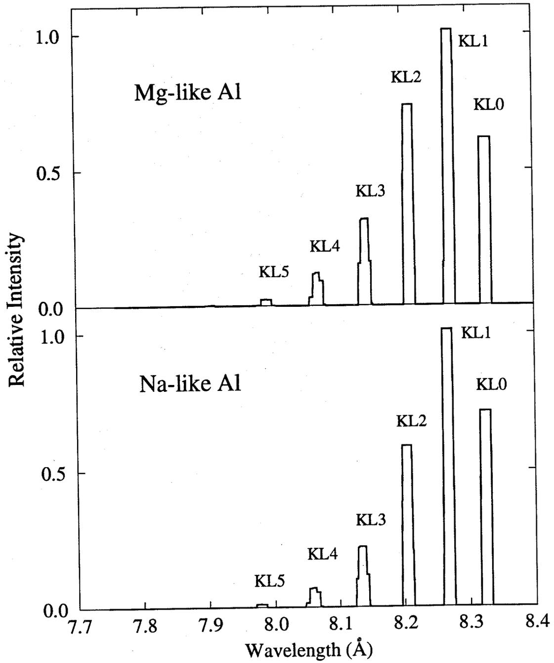
Figure 3. Computed Al  $K_{\alpha}$  satellite lines for Mg- and Na-like Al ions by 9 MeV  $\text{Li}^{+3}$  bombardment.
