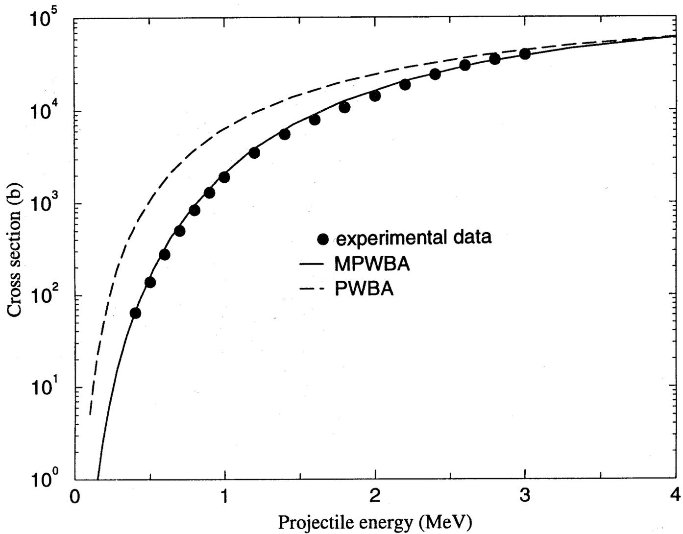
Figure 1. Al K-shell ionization cross sections by He<sup>2+</sup> bombardment. A comparison of PWBA and MPWBA results with experimental data (Richard et al. 1973).
