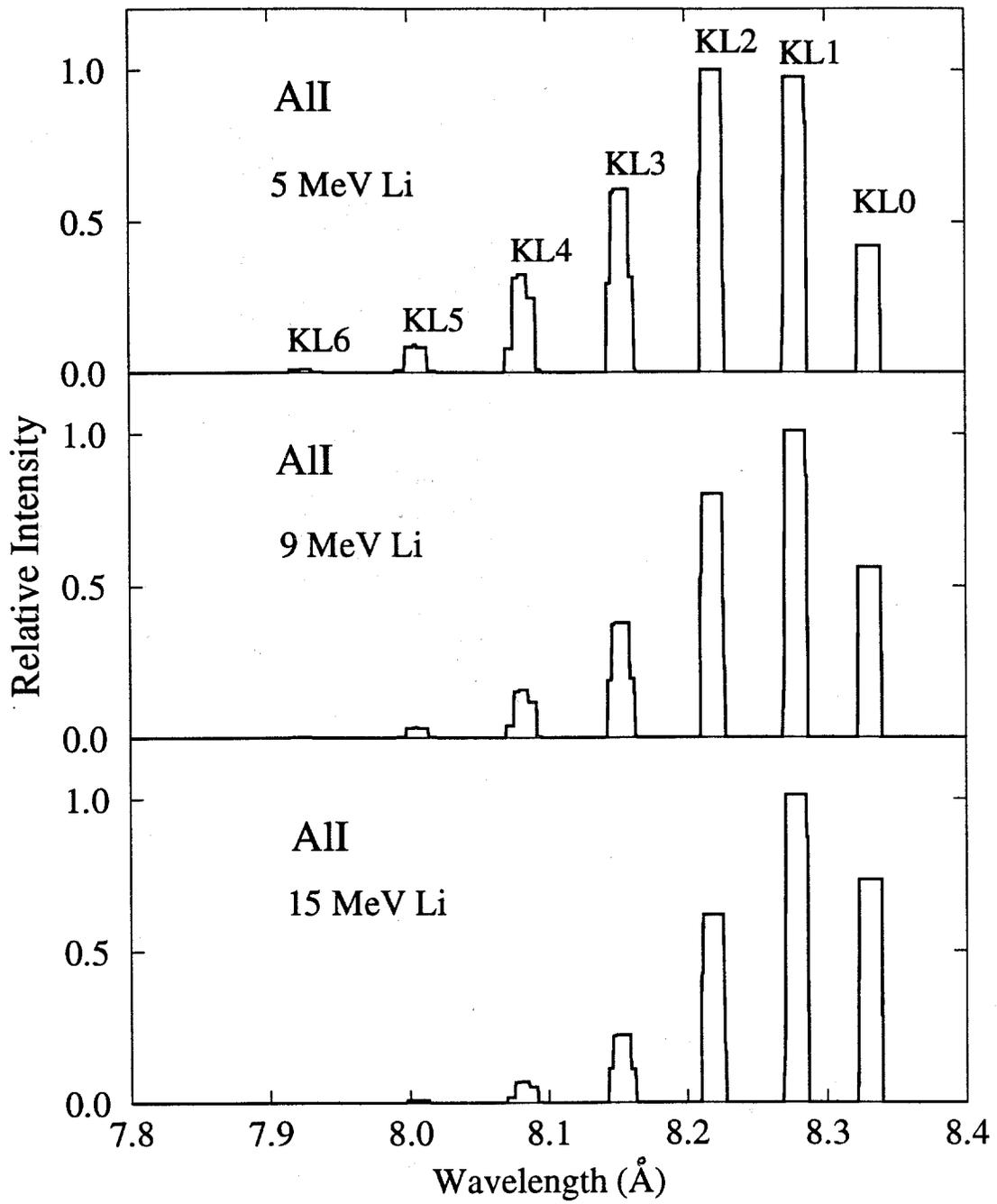
Figure 6. Computed Al  $K_{\alpha}$  satellite lines for neutral Al and B-like Al ions by 5, 9, and 15 MeV  $\text{Li}^{+3}$  bombardment.
