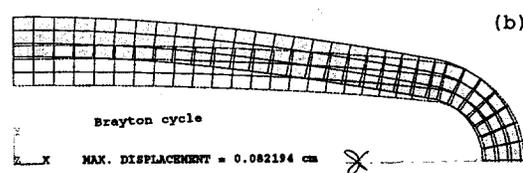
Fig. 6. Displacement of the first wall at midplane.
