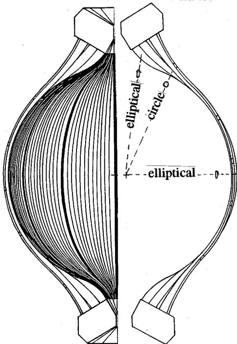
Fig. 2. Cross section of the first wall assembly showing the cross section of the first wall coolant tubing.
