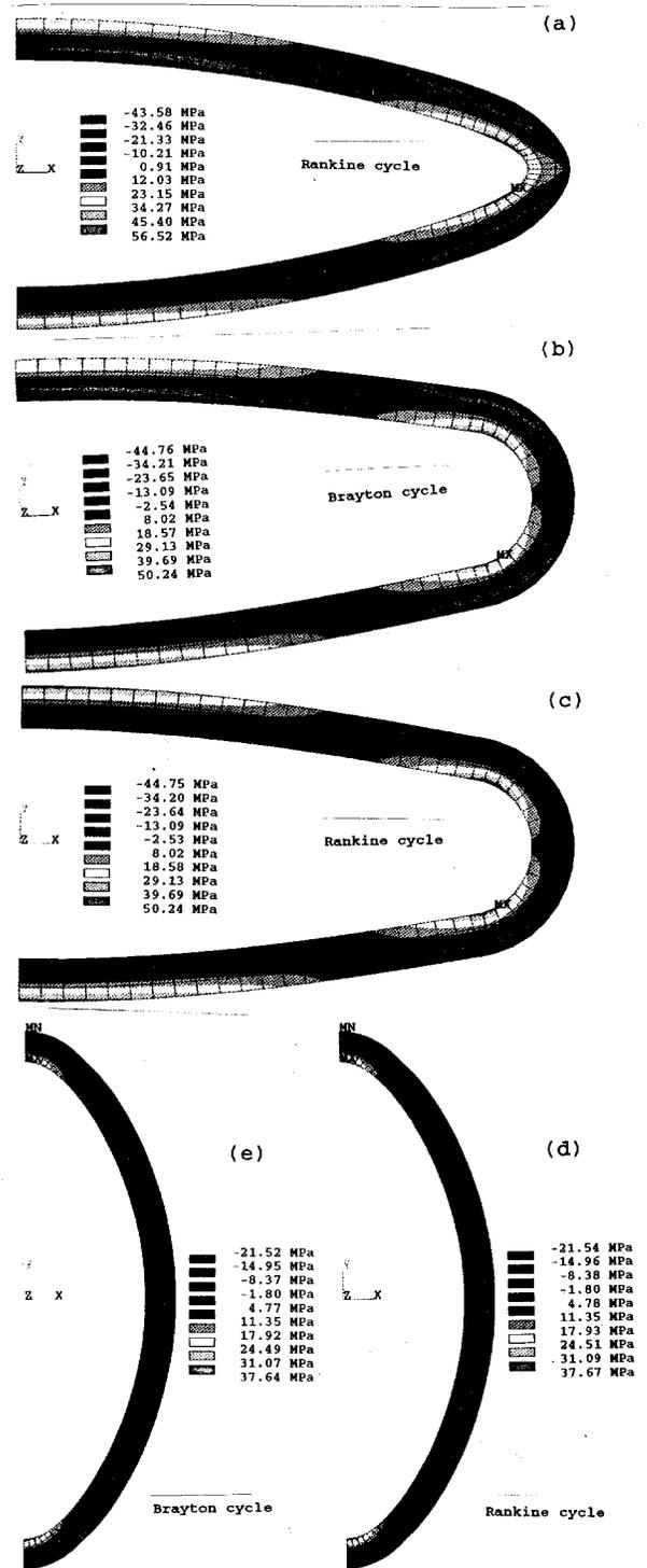
Fig. 4. Stress distribution normal to the fibers of the first wall at the midplane (a,b&c) and at the lower extremity (d&e) due to static and thermal loads (internal gas pressure = 1.5 atm).
