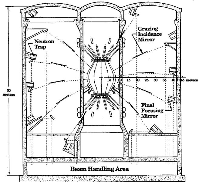
Fig. 1. SIRIUS-P reactor building showing the laser beams and the reactor cavity.
