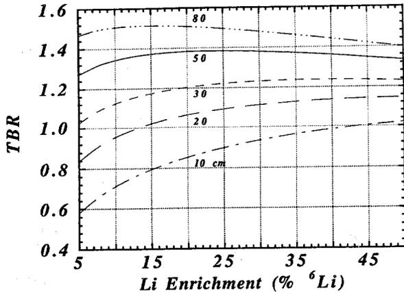
Fig. 1. Effect of Li enrichment on TBR for different blanket thickness.
