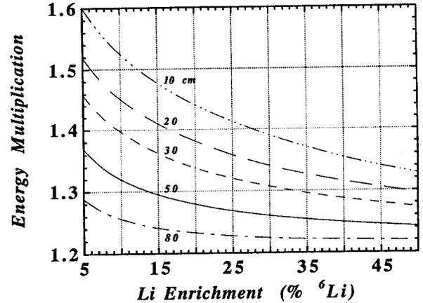
Fig. 2. Effect of Li enrichment on  $M$  for different blanket thickness.
