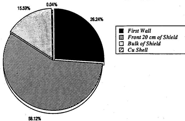
Fig. 5. Contribution to nuclear heating from different first wall and blanket zones.
