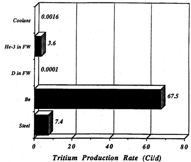
Fig. 8. Tritium production rate in the first wall and shield.
