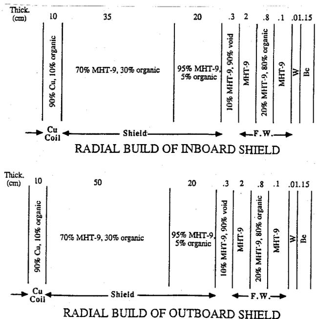
Fig. 4. Radial build of the reference first wall and shield.
