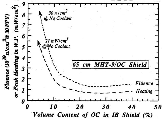
Fig. 2. Impact of organic coolant content on magnet damage.
