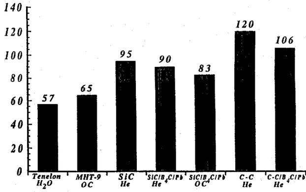
Fig. 1. Minimum inboard shield thickness (cm) required for different shield design options.
