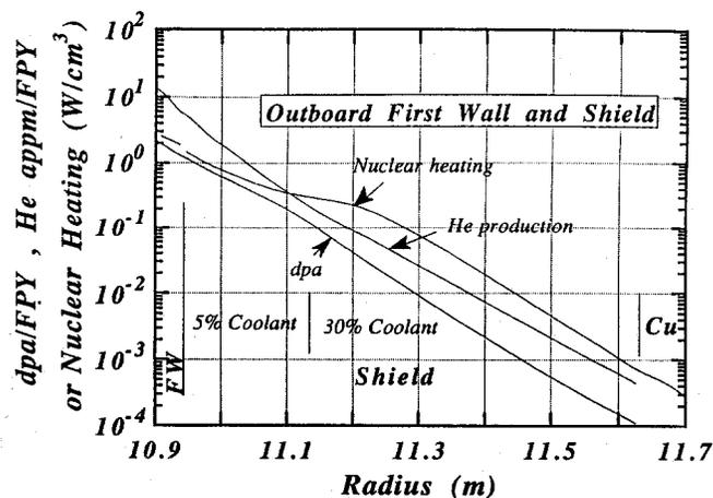
Fig. 6. Damage and nuclear heating profiles in the outboard FW and shield.
