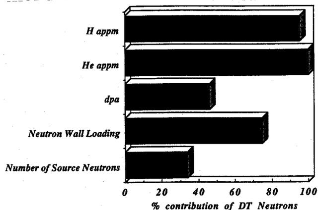
Fig. 7. Contribution of DT neutrons to FW damage parameters.
