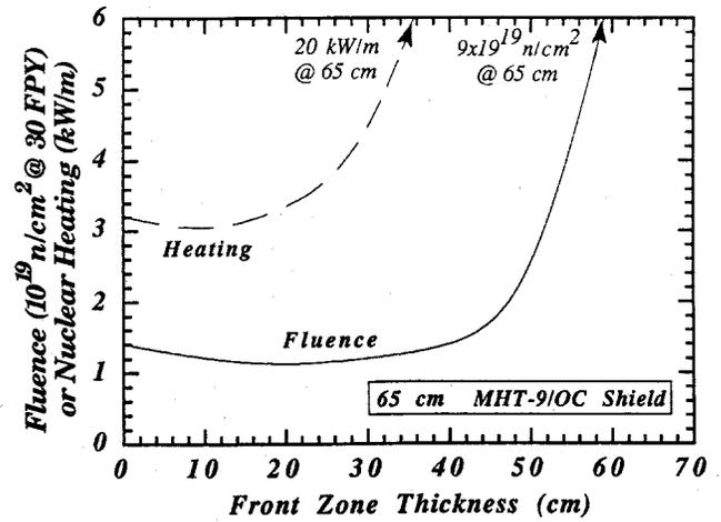
Fig. 3. Effect of varying thickness of the 5% OC front layer of shield.
