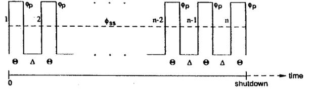
Fig. 1. Relation between the neutron flux during pulsed irradiation and the equivalent steady state flux.
