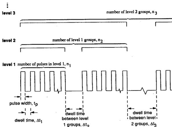
Fig. 4. Relation between various levels of regular pulse groupings during pulsed/intermittent operation.
