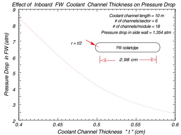
Figure 8. The effect of the first wall coolant channel thickness on the pressure drop in the first wall alone.
