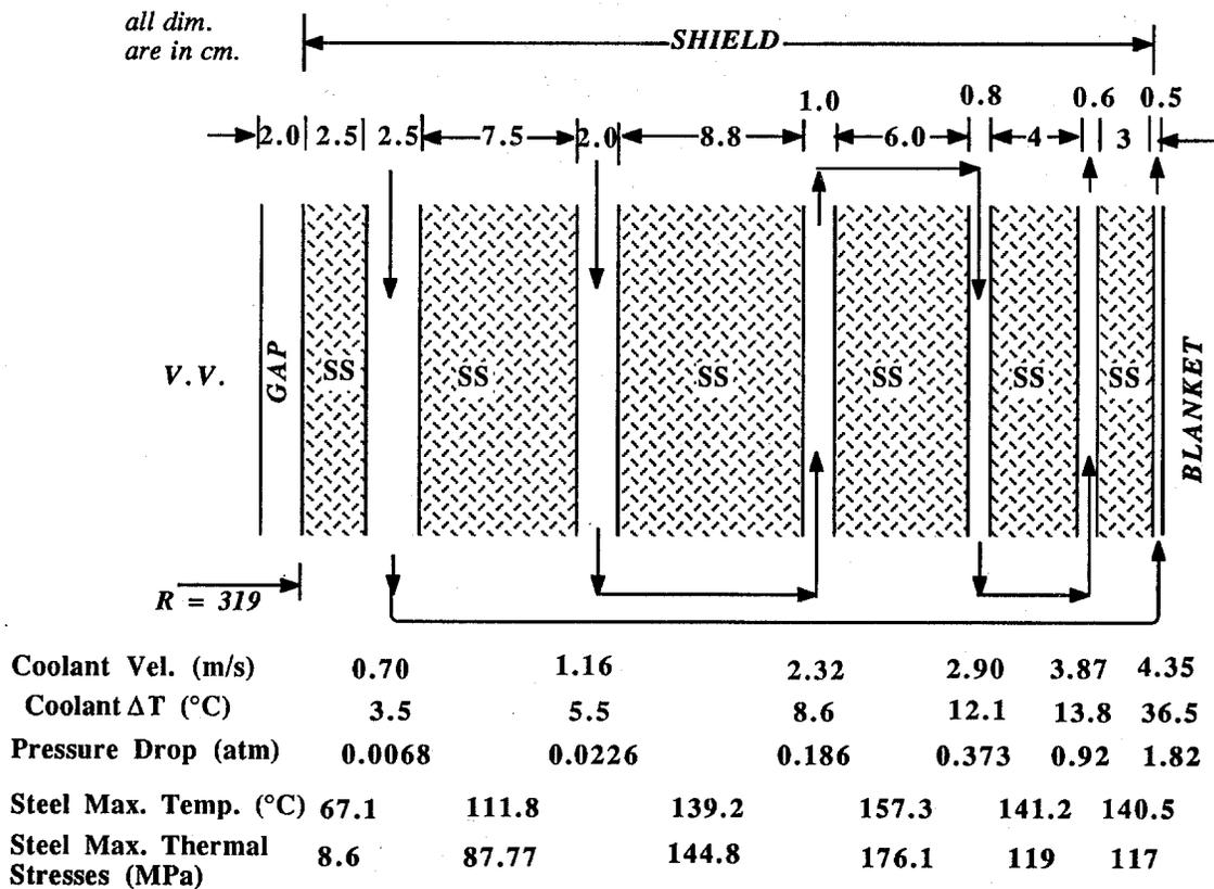
Figure 4. A schematic of the radial build of the inboard blanket
