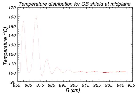
Figure 11. The temperature distribution for the outboard shield at midplane.
