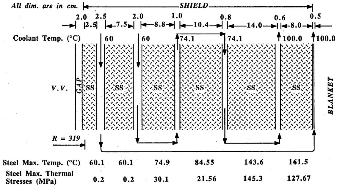
Figure 5. A schematic of the radial build of the inboard blanket
