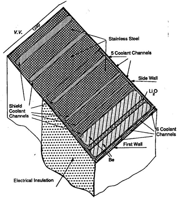
Figure 1. A schematic layout for 1/96 (one sector) of the inboard blanket and shield.
