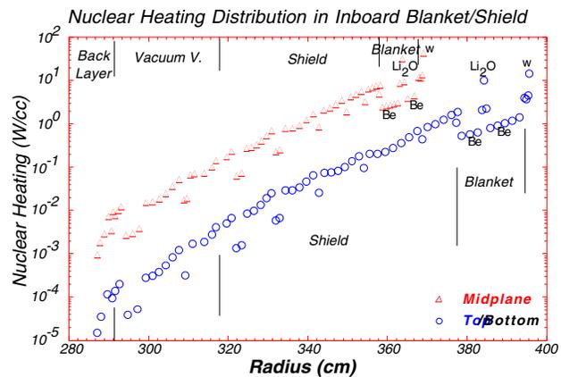
Figure 3. Nuclear heating distribution at the midplane and the top of the inboard blanket/shield.
