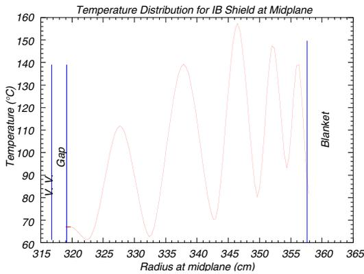
Figure 6. The temperature distribution for the I/B shield at the midplane of ITER.
