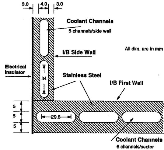
Figure 2. A schematic of the first wall and side wall coolant channels.
