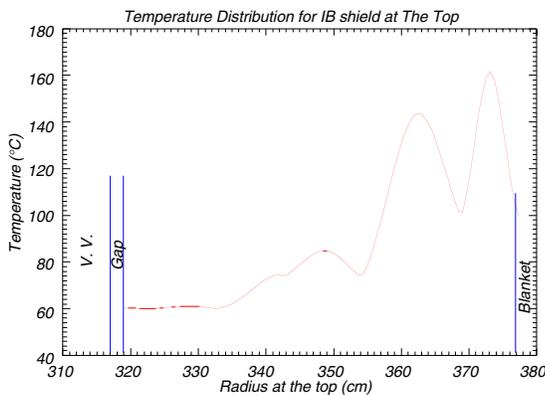
Figure 7. The temperature distribution for the I/B shield at the top of ITER.
