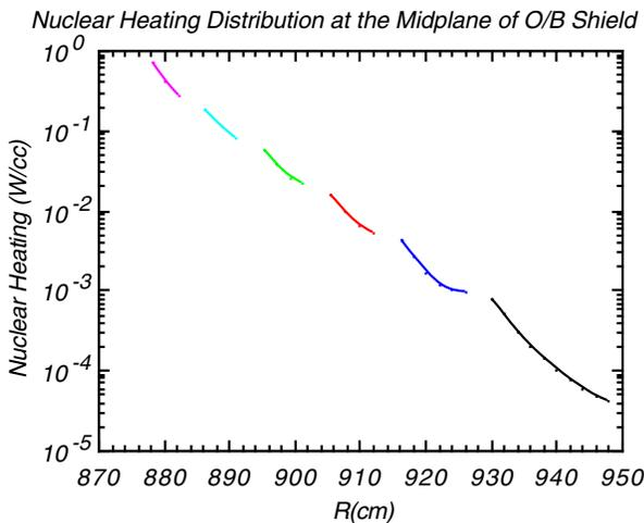
Figure 10. The nuclear heating for the outboard blanket/shield at midplane.
