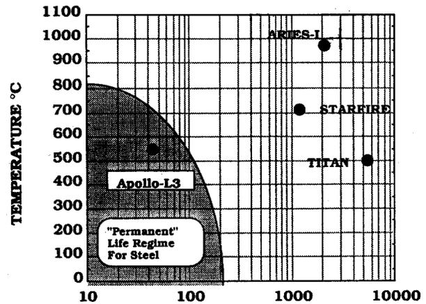
Figure 7. Permanent first walls are only possible for D-He3 reactors.
