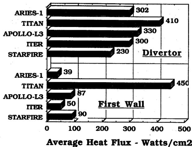
Figure 5. Heat fluxes in D-He3 reactors are comparable to DT fusion devices.
