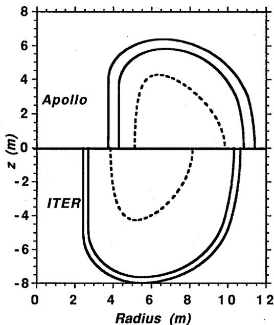
Figure 1b. Comparison of plasma shape and volume in Apollo-L3 with that in ITER.<sup>12</sup>
