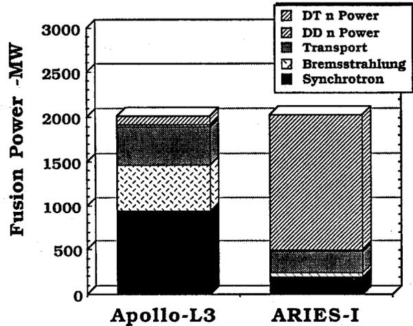
Figure 3. Comparison of energy release mechanisms from the plasma in a typical D-He3 (Apollo-L3) and a DT (ARIES-I) power plant.
