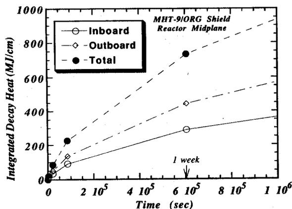
Figure 8. Afterheat in the Apollo-L3 shield after full lifetime exposure. Note this is the amount generated and energy remaining in structure depends on energy loss mechanisms.
