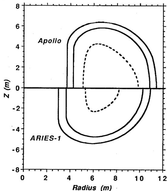
Figure 1a. Comparison of plasma shape and volume in Apollo-L3 with that in ARIES-1.<sup>7</sup>
