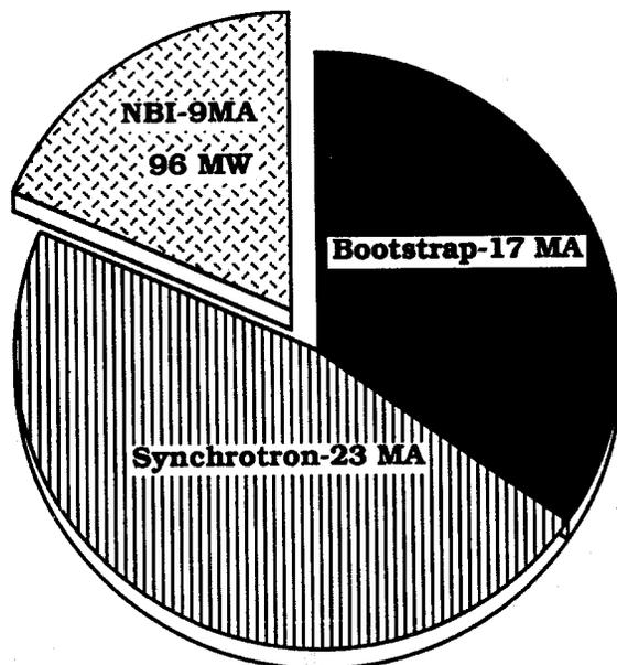
Figure 4. Current drive mechanisms in Apollo-L3.
