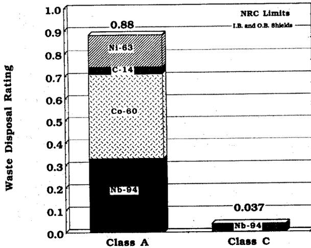
Figure 9. The low activation ferritic alloys qualify as low level class A wastes. The waste disposal rating for class C is 0.037 which is more than a factor of 25 below the class C limit.
