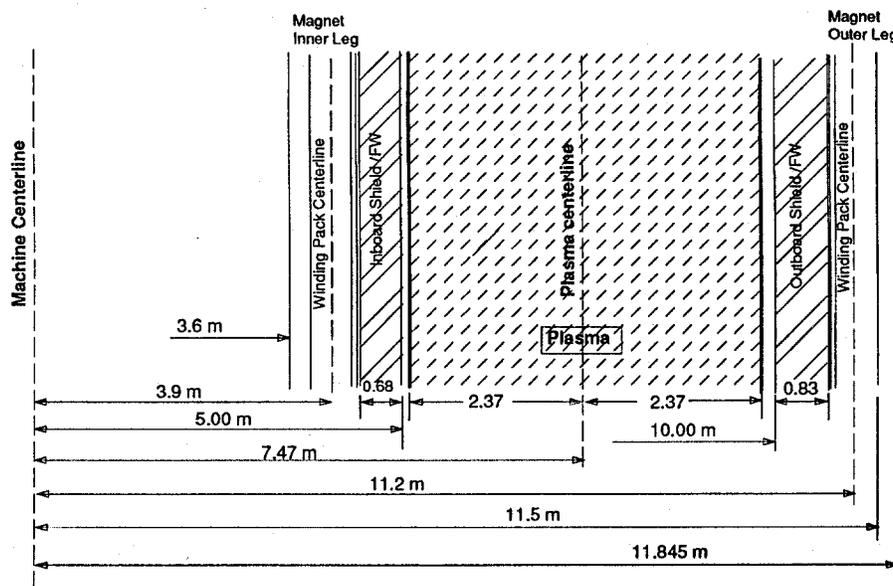
Figure 6. Schematic of Apollo-L3 first wall and shield at the midplane.
