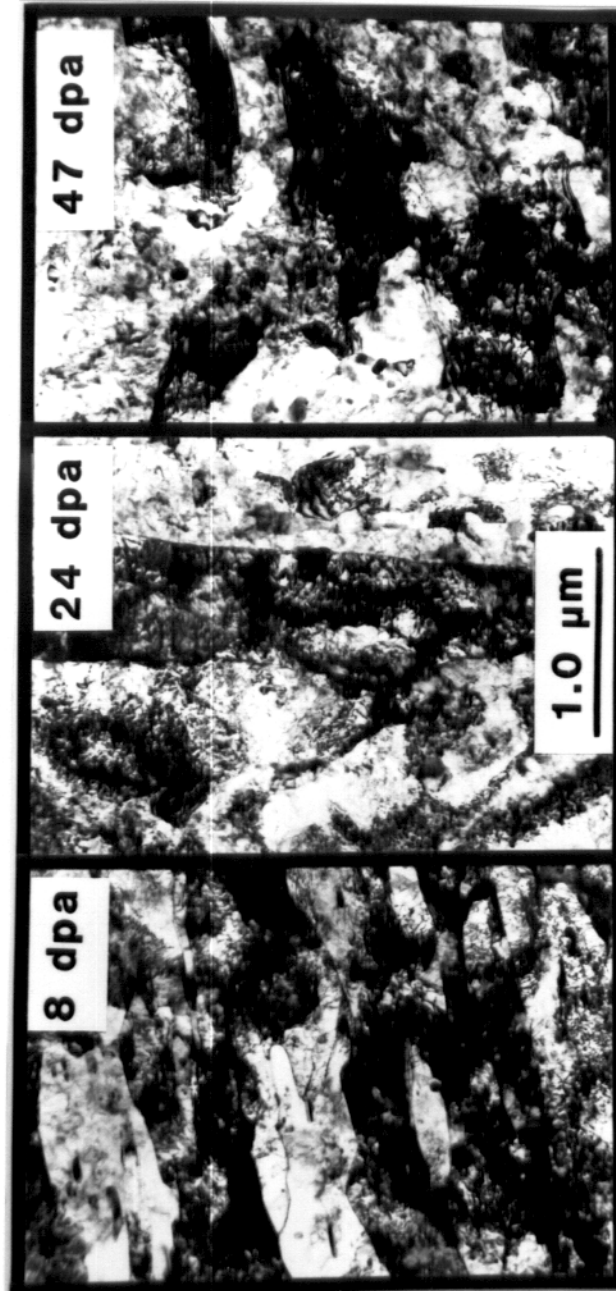
Figure 6.7. TEM micrographs of L9 ion-irradiated at 450C.
