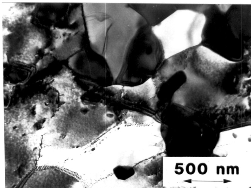
Figure 6.4. L9 neutron irradiated to 48 dpa at 520°C. The smooth grains are chi.
