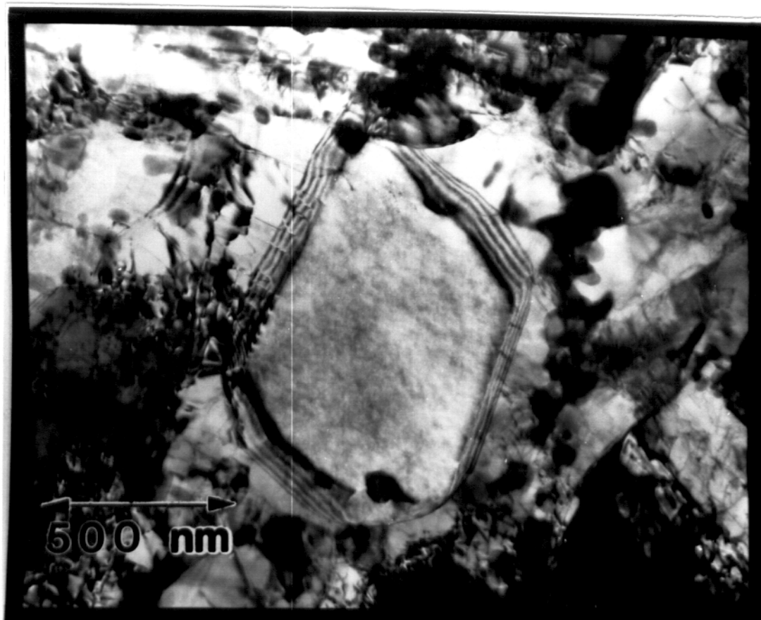
Figure 5.13. Delta Ferrite in L9 aged for 5000 hours at 600°C.
