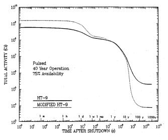
Fig. 4. Effect of Low Activation Structure on Total Activity in LIBRA Chamber.
