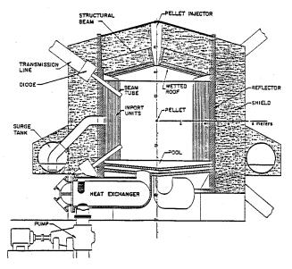
Fig. 1. Cross Section of Target Chamber.
