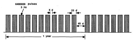
Fig. 2. Pulse Sequence Used in the LIBRA Activation Calculations.
