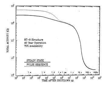
Fig. 3. Effect of Pulse Sequence on Total Activity in LIBRA Chamber.
