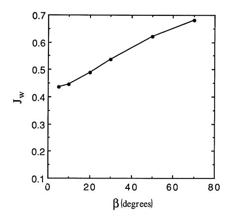
Figure 10: Neutral helium current to the plate versus  $\beta$  ( $z_{max}$  = 25 cm,  $L_p = 1.575$  cm,  $F_A = 0.25$  and  $\theta_w = 90^\circ$ ).
