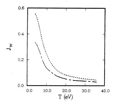
Figure 8: Neutral helium current to the plate versus temperature. (---) no reflection at the plate, (---) includes reflection at the plate.
