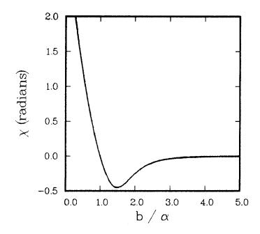
Figure 4: Classical deflection function versus normalized impact parameter (center of mass energy = 5.79567 eV).
