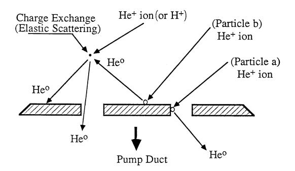
Figure 2: Recycling at the target plate.
