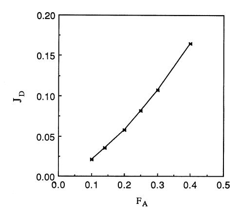
Figure 11: Neutral helium current to the pump duct versus  $F_A$  ( $z_{max} = 25$  cm,  $\theta_w = 90^\circ$  and  $\beta = 10^\circ$ ).
