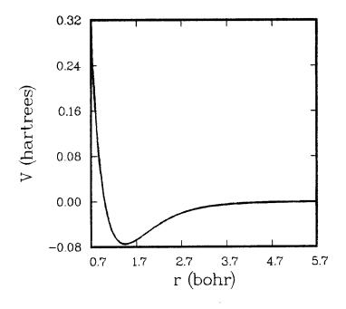
Figure 3: Wolniewicz potential versus proton-helium atom separation distance.
