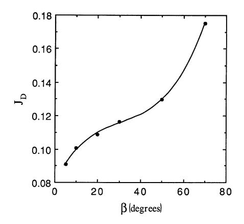
Figure 14: Neutral helium current to the pump duct versus  $\beta$  ( $z_{max} = 25$  cm,  $L_p = 1.575$  cm,  $F_A = 0.25$  and  $\theta_w = 90^\circ$ ).
