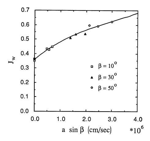
Figure 16: Neutral helium current to the plate versus  $a \sin \beta$   $(n_p = 1 \times 10^{14} \text{ cm}^{-3} \text{ and } T_i = 4 \text{ eV}).$
