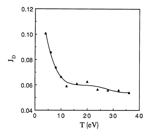
Figure 15: Neutral helium current to the pump duct versus T  $(n_p = 1 \times 10^{14} \text{ cm}^{-3})$ .
