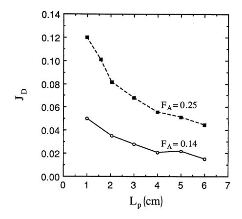
Figure 12: Neutral helium current to the pump duct versus  $L_p$  ( $z_{max} = 25$  cm,  $\theta_w = 90^\circ$  and  $\beta = 10^\circ$ ).
