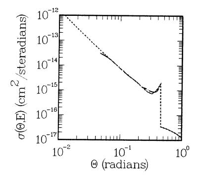
Figure 5: Classical differential elastic scattering cross section (center of mass energy = 5.79567 eV), --- our results, --- Helbig results.
