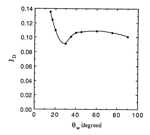
Figure 13: Neutral helium current to the pump duct versus  $\theta_w$  ( $z_{max} = 25$  cm,  $L_p = 1.575$  cm,  $F_A = 0.25$  and  $\beta = 10^{\circ}$ ).
