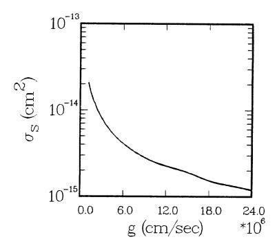
Figure 6: Total elastic scattering cross section versus helium-proton relative speed.
