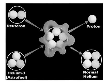
Figure 3. The Astrofuel fusion reaction, which releases 18.4 MeV of energy per event.
