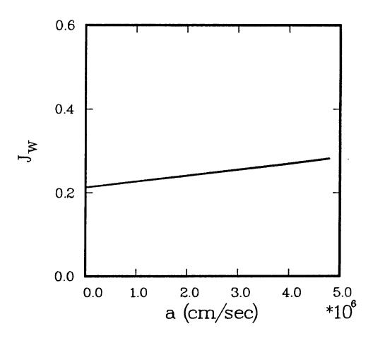
Figure 11: Neutral helium current to the plate versus ion flow speed.
