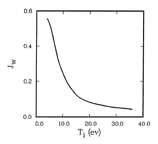
Figure 9: Neutral helium current to the plate versus temperature.
