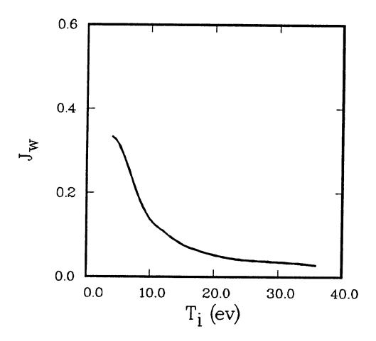
Figure 10: Neutral helium current to the plate versus temperature.
