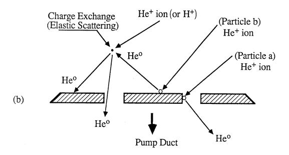
Figure 1: (a) TIBER-II's previously proposed divertor with its flat vented plates (from LLNL/TIBER 86-25). (b) Recycling at the plate.
