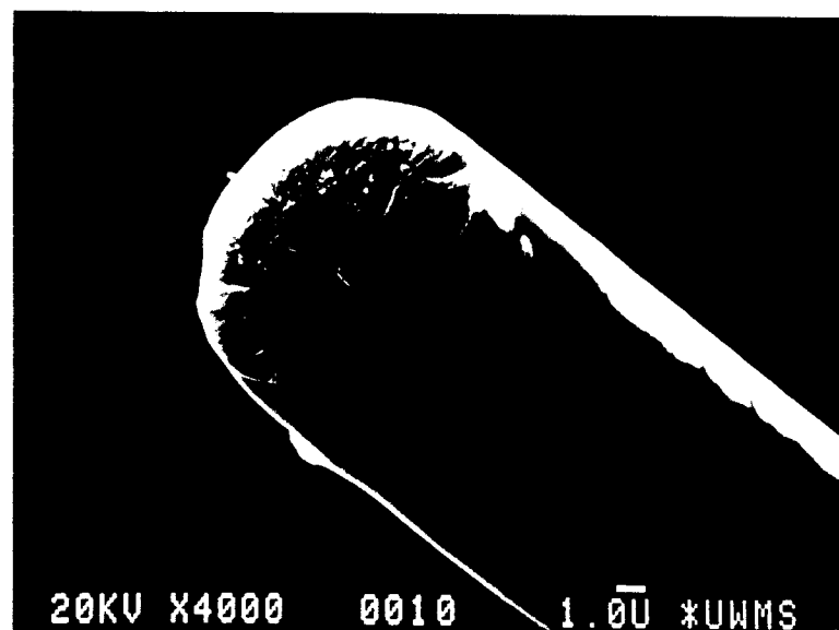
Fig. A.1-6. SEM micrograph of filament tensile failure.
