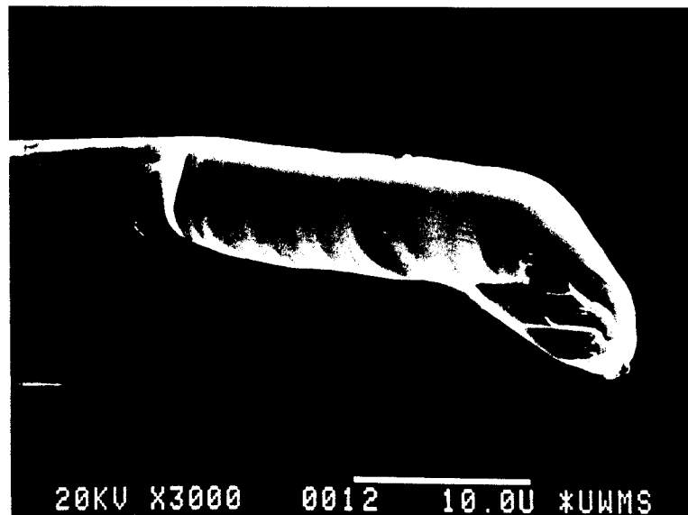
Fig. A.1-11. Fatigue fiber fracture at 13,700 cycles for \sigma_m/\sigma_f = 40\% , \sigma_a/\sigma_f = 20\% .
