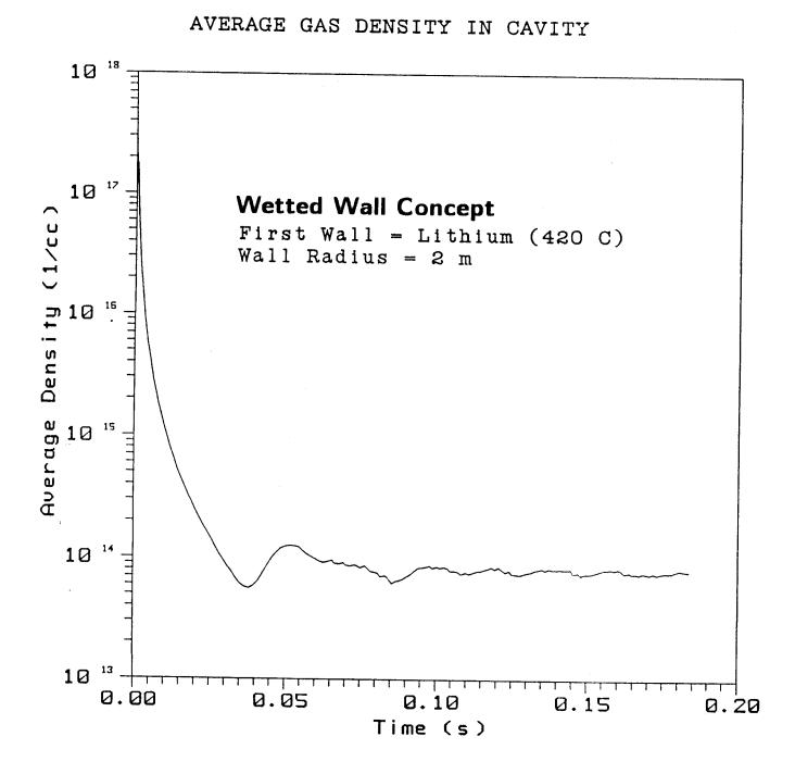
Fig. 8. Average Vapor Density in a Wetted-Wall Target Chamber Versus Time.
