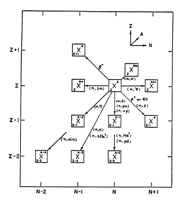
Figure 2.1. Transmutation products by neutron reaction and by radioactive decay.
