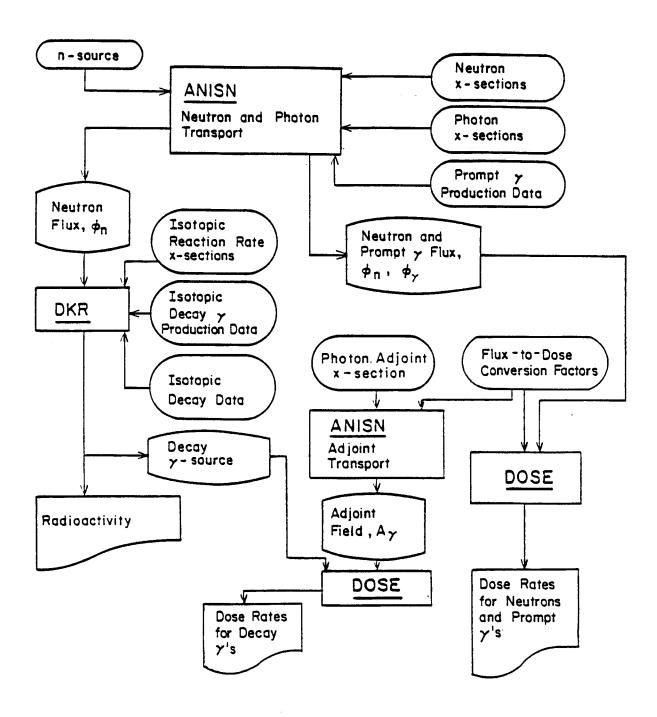
Figure 3.2. Flowchart for the calculation of dose rates using the adjoint scheme.
