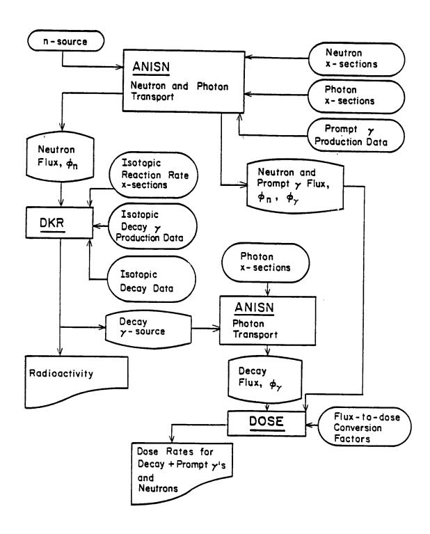
Figure 3.1. Flowchart for the calculation of dose rates using the forward scheme.
