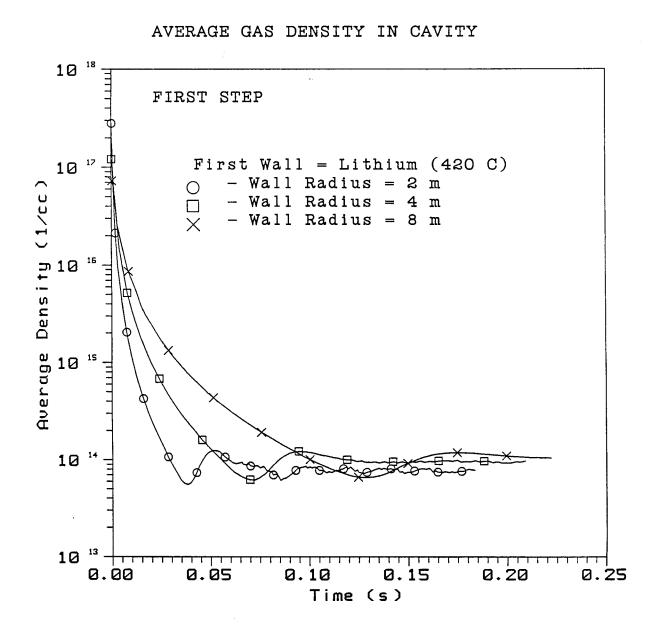
Fig. 2. Average number density in cavity versus time for various target chamber radii. The bulk temperature of the wall is  $420^{\circ}$ C and there are initially 150 gm of vaporized material.
