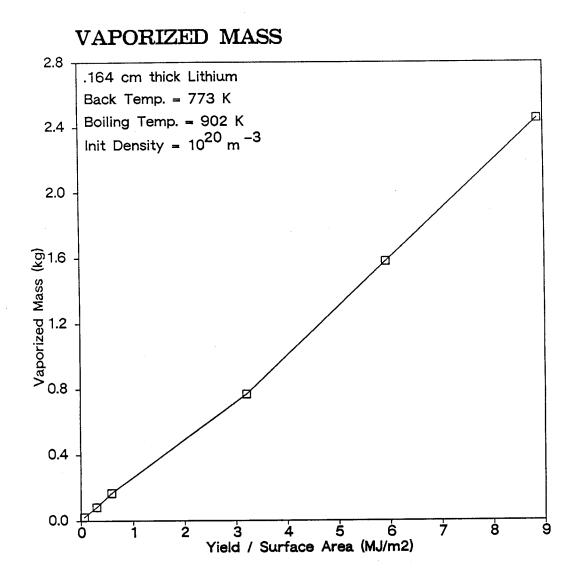
Fig. 1. Vaporized mass as a function of the yield per unit area. The cavity radius is 2 meters, the first wall is lithium and the HIBALL x-ray spectrum is used.
