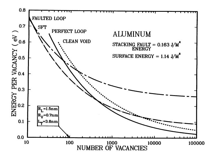
Figure 3. Calculated specific energies of vacancy clusters in pure aluminum.
