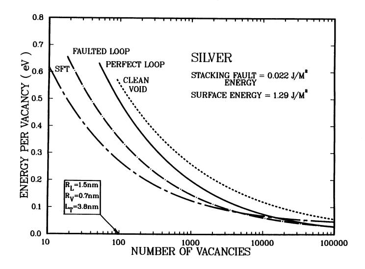
Figure 2. Calculated specific energies of vacancy clusters in pure silver.
