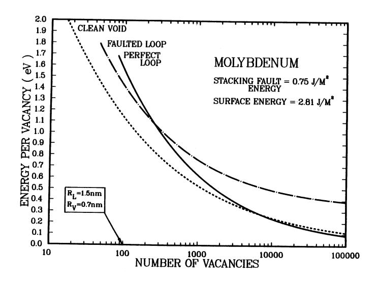
Figure 8. Calculated specific energies of vacancy clusters in pure molybdenum.
