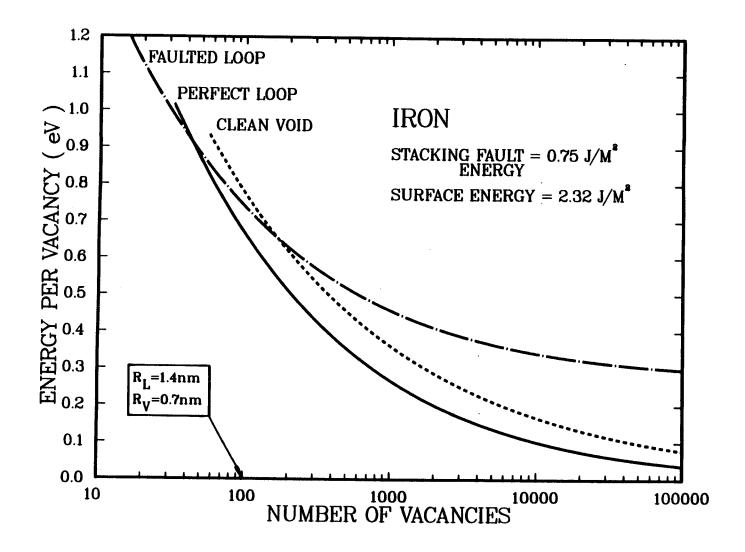
Figure 7. Calculated specific energies of vacancy clusters in pure iron (bcc).
