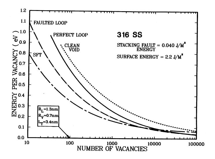
Figure 6. Calculated specific energies of vacancy clusters in 316 stainless steel.
