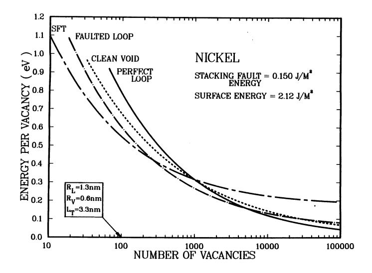
Figure 5. Calculated specific energies of vacancy clusters in pure nickel.
