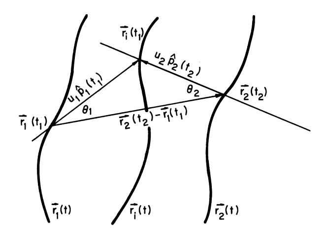
Fig. 2. Determination of the curve of intersection  $\vec{r}_1$  of two developable surfaces. The directrix curves for the two surfaces are  $\vec{r}_1$  and  $\vec{r}_2$ ; the respective unit ruling vectors are  $\hat{p}_1$  and  $\hat{p}_2$ .
