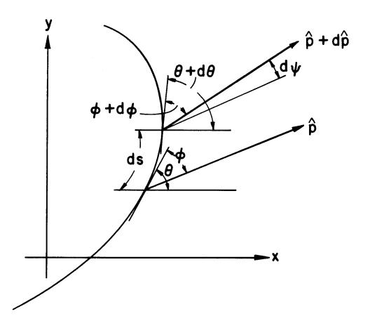
Fig. 4. Determination of the position and orientation of the directrix curve and rulings in the developed surface.
