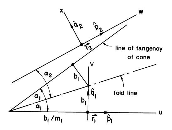
Fig. 5. Determination of the line of tangency of cone segments on successive tangent planes to a developable surface.
