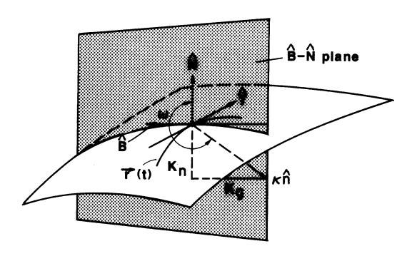
Fig. 3. Geometrical interpretation of normal and geodesic curvature.
