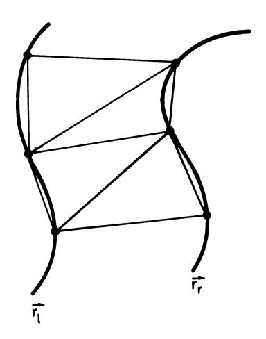
Fig. 6. Approximation of a general ruled surface by triangular elements.
