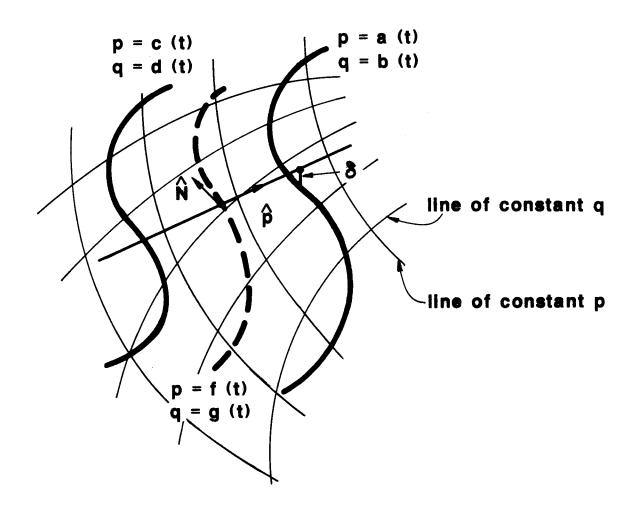
Fig. 1. Approximation of a general surface by the envelope of tangent planes to the surface along the curve p=f(t), q=g(t). The distance  $\delta$  is a measure of the deviation of the ideal and approximate surfaces at a boundary line.
