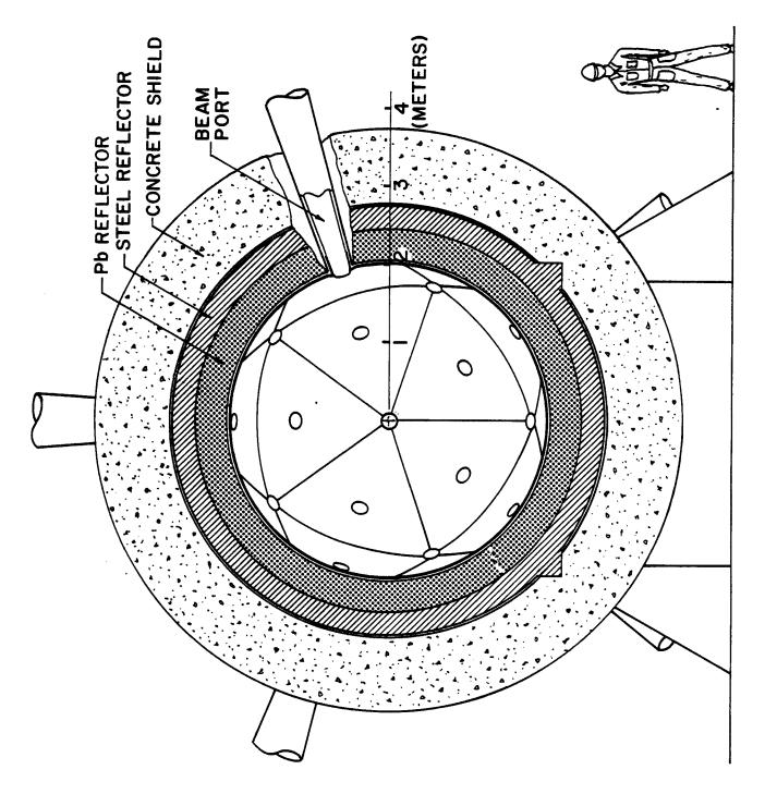
Fig. 1. SIRIUS-M cavity, reflector and shield.
