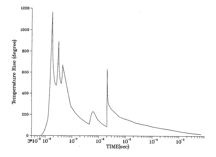
Fig. 7. Temperature rise in graphite tiles in SIRIUS-M for base case.
