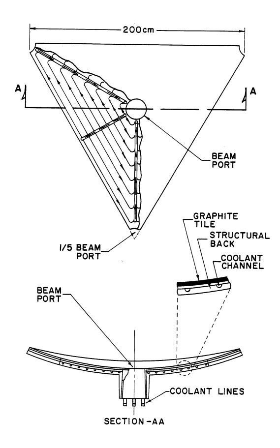
Fig. 2. Actively cooled graphite-faced tile.
