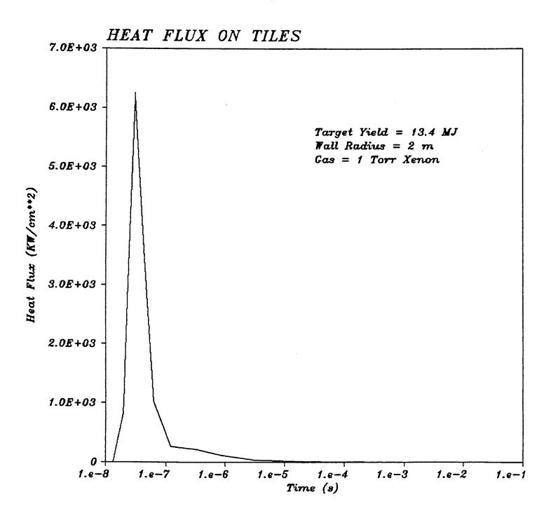
Fig. 6. Radiation heat flux on the first wall of the SIRIUS-M target chamber.
