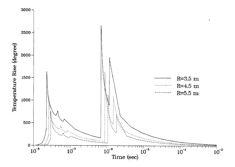
Fig. 4. Temperature rise at the front surfaces of the FW for a cavity radius of 3.5, 4.5 and 5.5 m, with a steady state temperature of  $500^{\circ}$ K.
