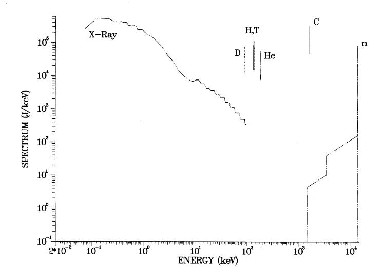
Fig. 3. X-ray, ion and neutron spectra for the SIRIUS-M target.
