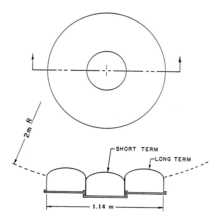
Fig. 8. Geometrical configuration of the test module.
