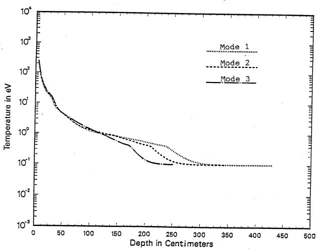
Fig. 7. Temperature rise in Xe gas due to energy deposition of ions.
