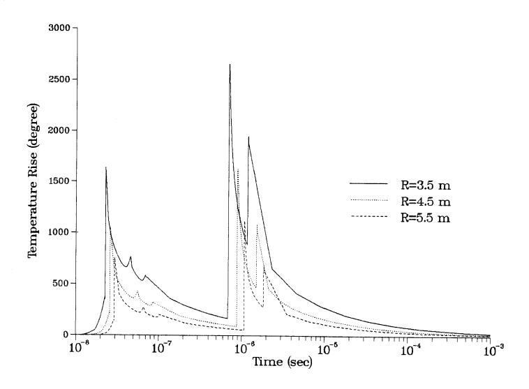
Fig. 4. Temperature rise at the graphite first wall front surface for cavity radii of 3.5, 4.5 and 5.5 m, with a steady state temperature of 500°K.
