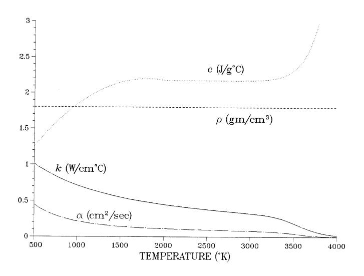
Fig. 3. Graphite thermal properties as a function of temperature: density  $\rho$ , conductivity k, diffusivity  $\alpha$ , specific heat c.
