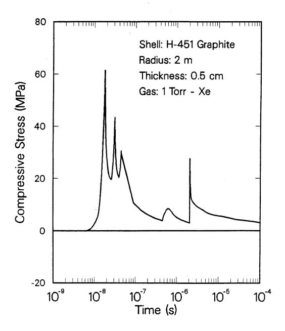
Fig. 12. SIRIUS-M graphite first wall thermal stress history.
