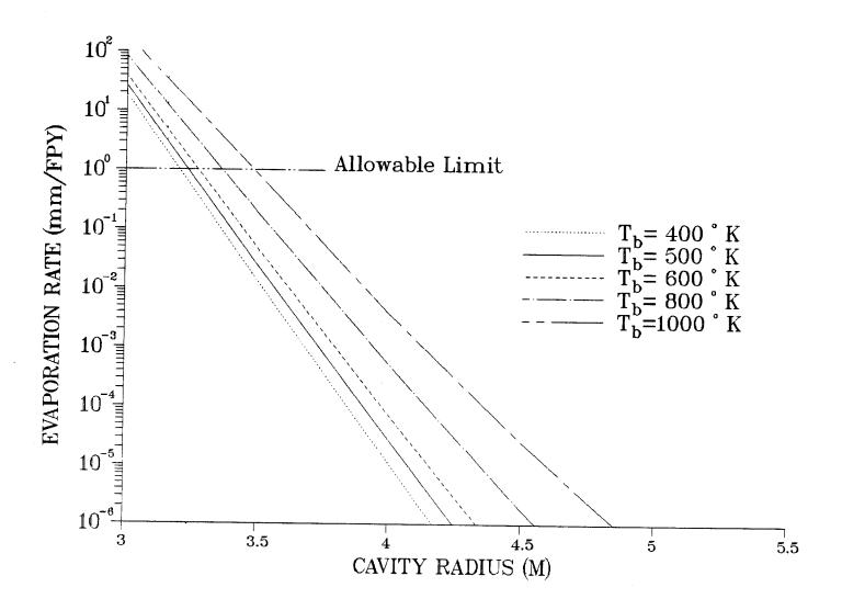
Fig. 6. Evaporation rate as a function of the cavity radius and steady state surface temperature.
