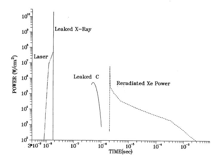
Fig. 9. Total heat flux on first wall including reflected laser, reradiated, and unabsorbed target x-rays and ions for base case.
