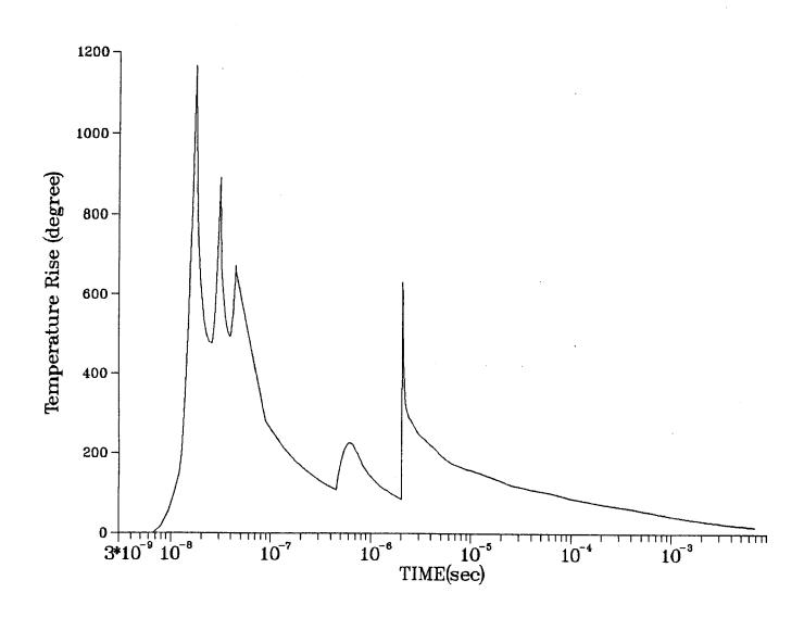
Fig. 10. Temperature rise in graphite first wall of SIRIUS-M base case.
