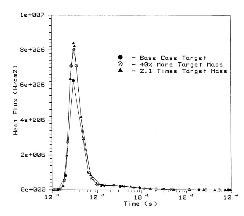
Fig. 8. Graphite first wall heat flux for various target designs.
