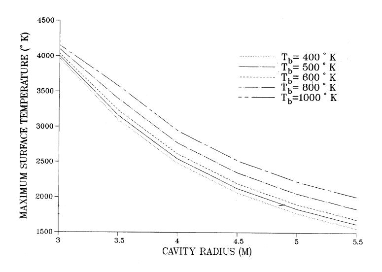
Fig. 5. The maximum surface temperature for various steady state temperatures and cavity radii.
