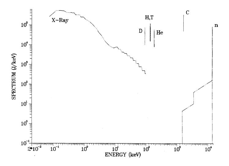
Fig. 1. X-ray, ion, and neutron spectra.
