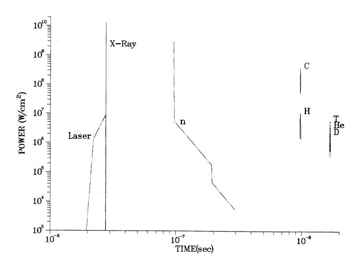
Fig. 2. Incident power on an unprotected wall (R = 5 m) due to x-rays, ions, neutrons and laser light reflected from the target.
