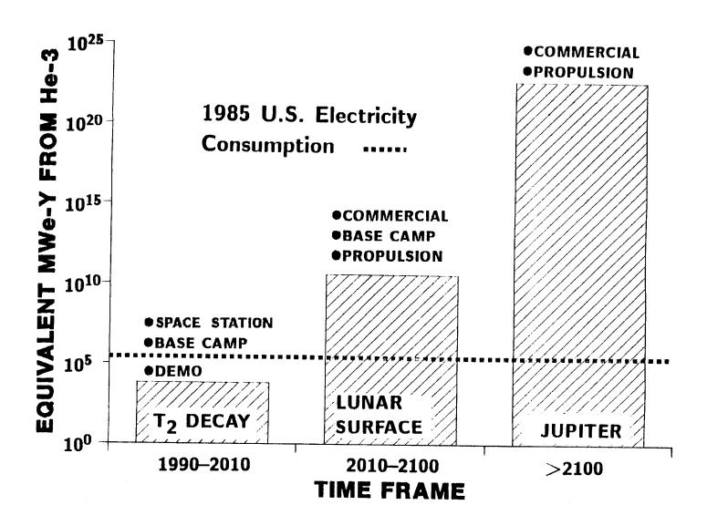
Fig. 4. Equivalent electrical energy content of He-3 sources.
