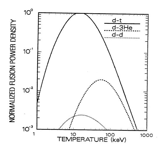
Fig. 2. Normalized fusion power density as a function of ion temperature for selected fusion fuels.
