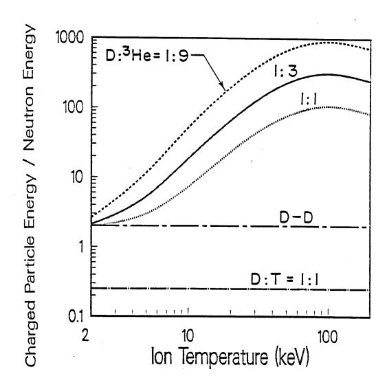
Fig. 1. Ratio of charged particle power to neutron power as a function of ion temperature for selected fusion fuels.
